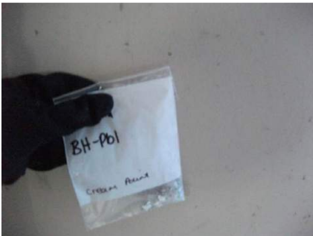
Photograph 27: Boat House Building – Lead-Based Cream Wall Paint
