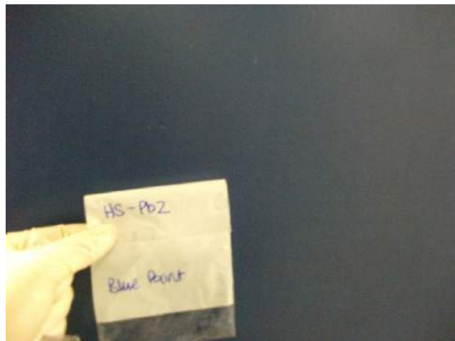
Photograph 18: Heated Storage Building – Lead-Based Blue Wall Paint
