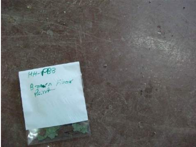
Photograph 25: Helicopter Hangar Building – Lead-Based Brown Floor Paint
