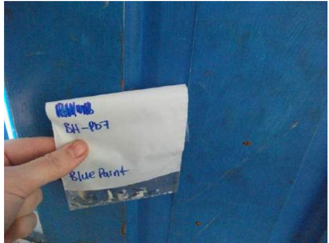
Photograph 30: Boat House Building – Lead-Based Blue Wall Paint
