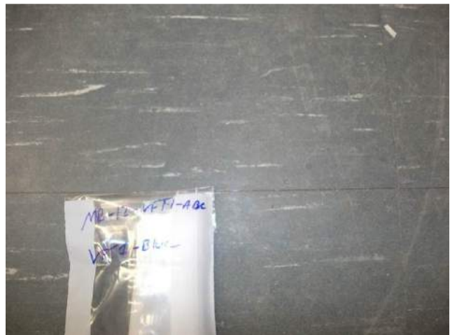
Photograph 4: Main Building – ACM (VFT1) Blue With White Streak 12" X 12" Vinyl Floor Tile
