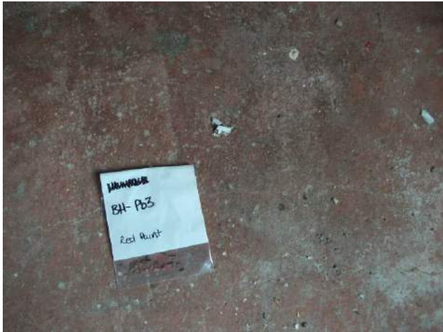
Photograph 29: Boat House Building – Lead-Based Red Floor Paint
