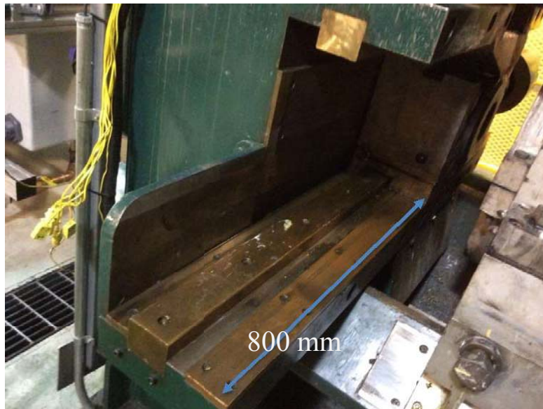
Figure 6. Stroke length of the die insertion system.
