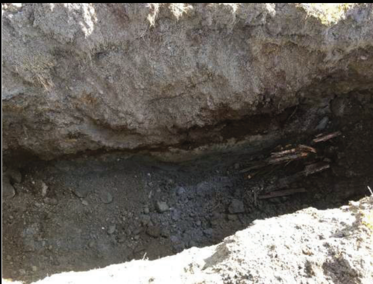
Photo 4: Looking into TP16-03, note the large amount of wood debris within the fill layer on the right side.
