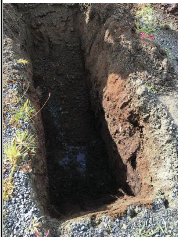
Photo 2: Looking into TP16-01, note fill near surface and the minor water seepage pooling at the bottom.
