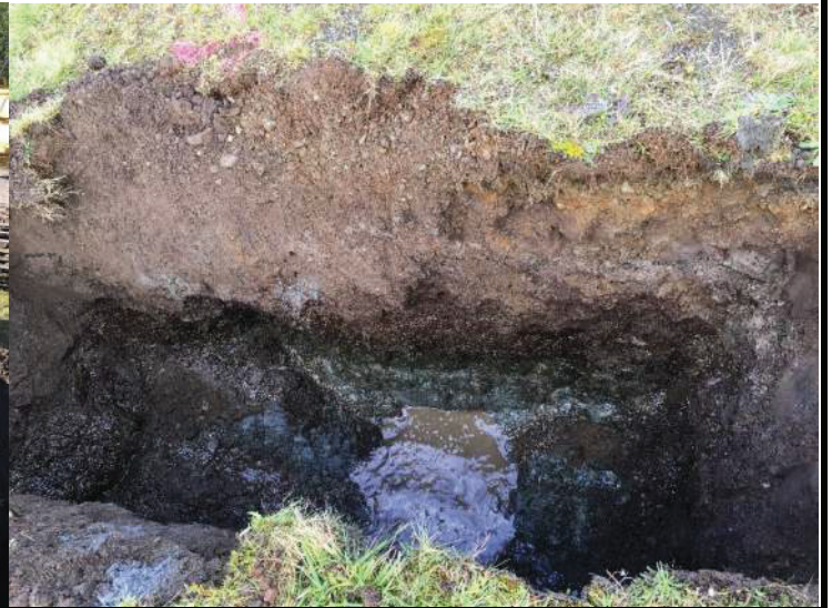
Photo 7: Looking into TP16-06, note large amount of pooling water.
