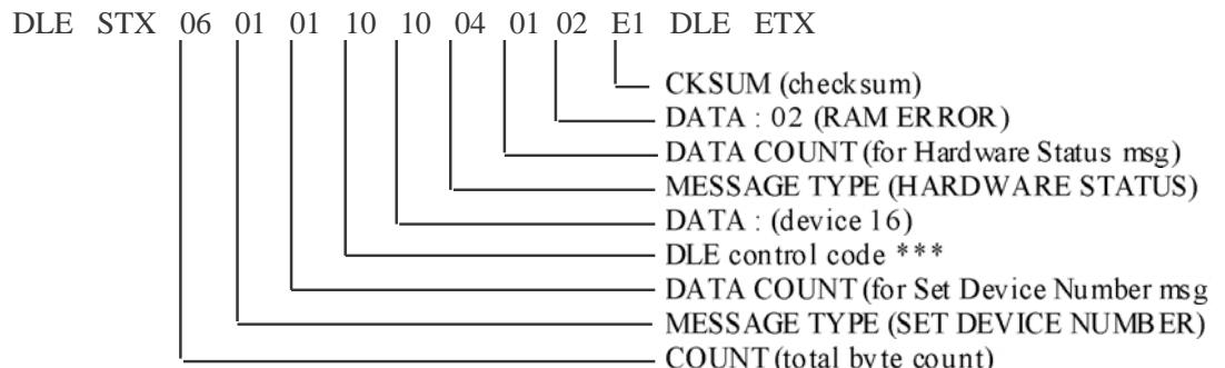
\*\*\* The DLE control code (10h) is inserted before the data value 10h.
