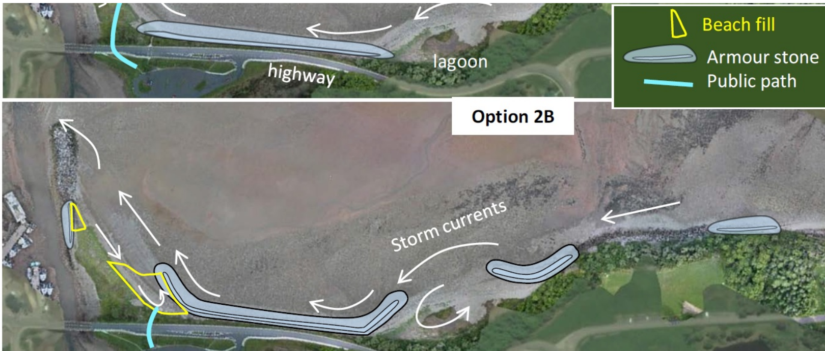
Figure 2. Option 2B – Boardwalk, Beach Fill, Curved Armour Stone Revetment and Breakwaters (CBCL Ltd 2017 - PCA Digital Files).
