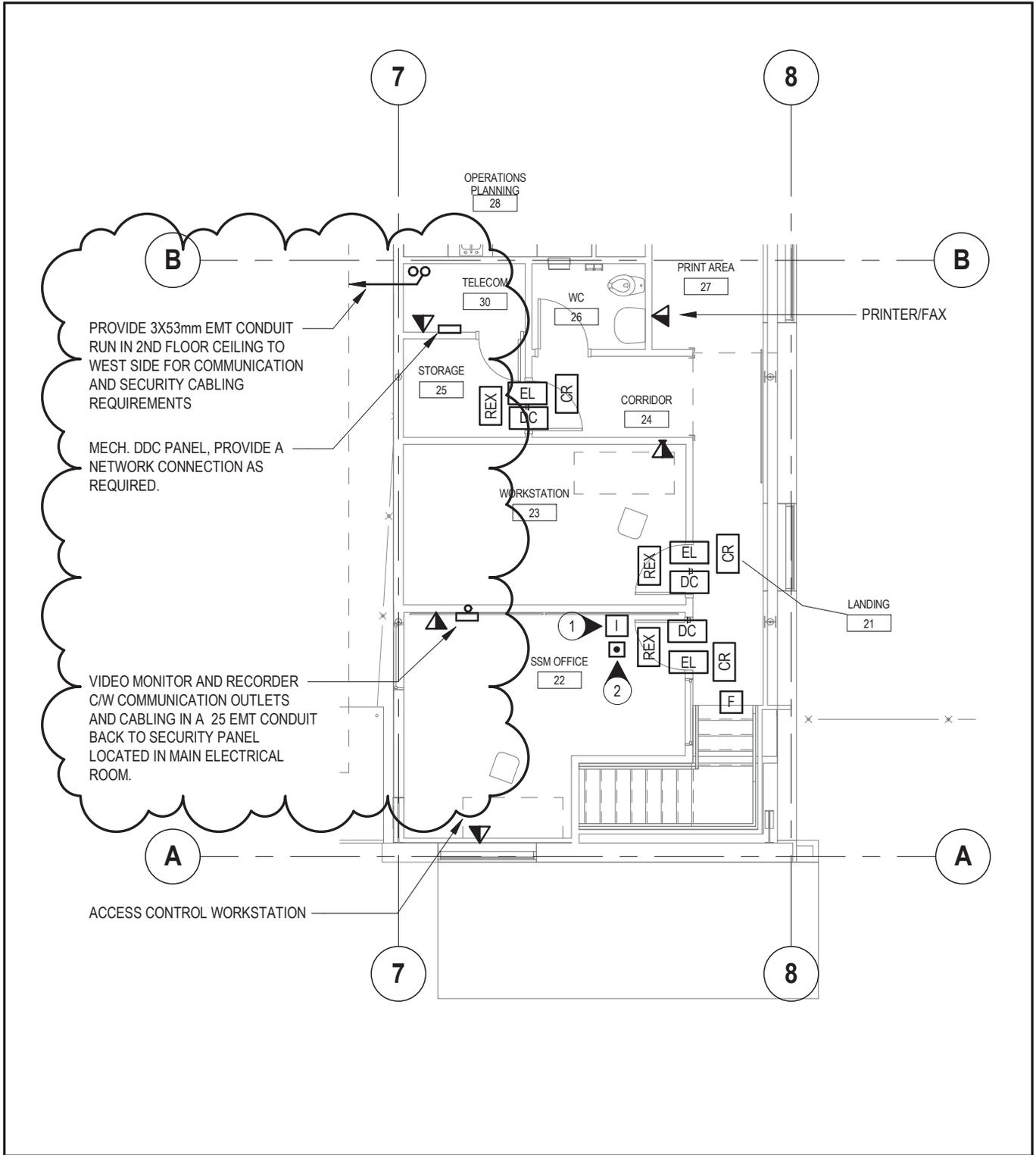
PROVIDE 3X53mm EMT CONDUIT RUN IN 2ND FLOOR CEILING TO WEST SIDE FOR COMMUNICATION AND SECURITY CABLING REQUIREMENTS
