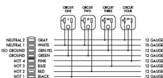
**NOTE:** The 4-circuit connection monument can utilize either of the above wiring schemes
