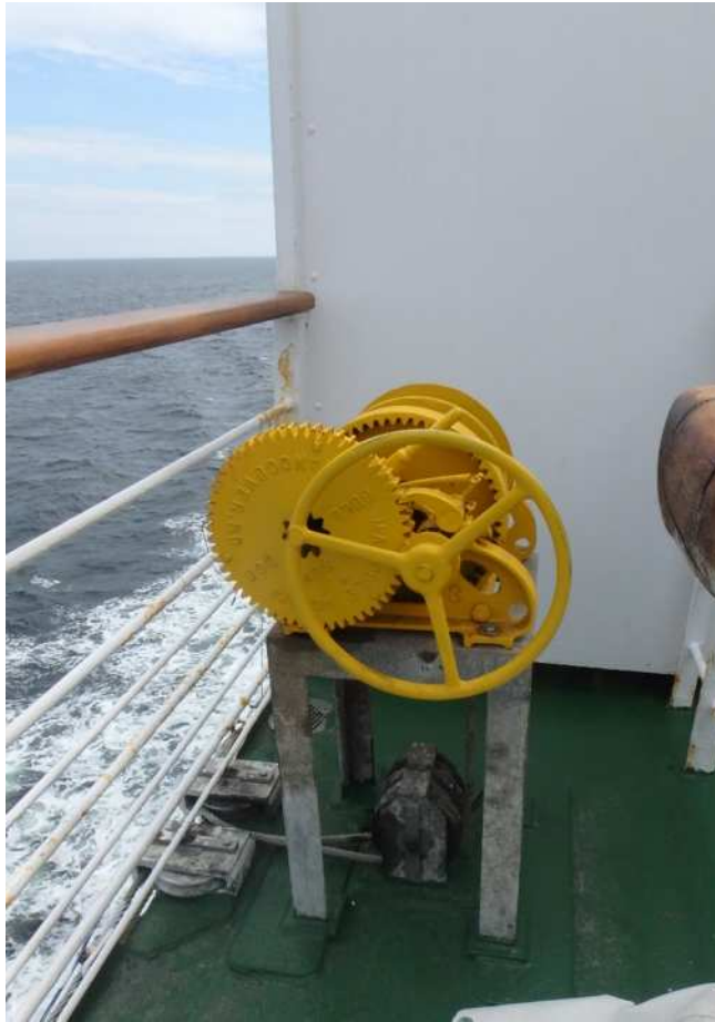
Figure 3: bowing winch with vertical & horizontal pulleys
