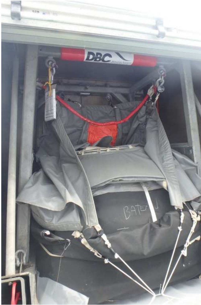
Figure 2: chute, with inboard door open
