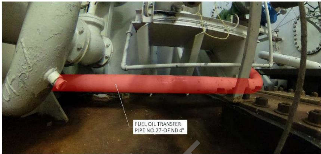
Figure 18 Fuel Oil transfer 27-OF, connection at bulkhead 138
