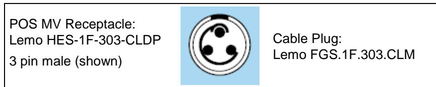
Figure 10: PWR Connector Pin Arrangement
