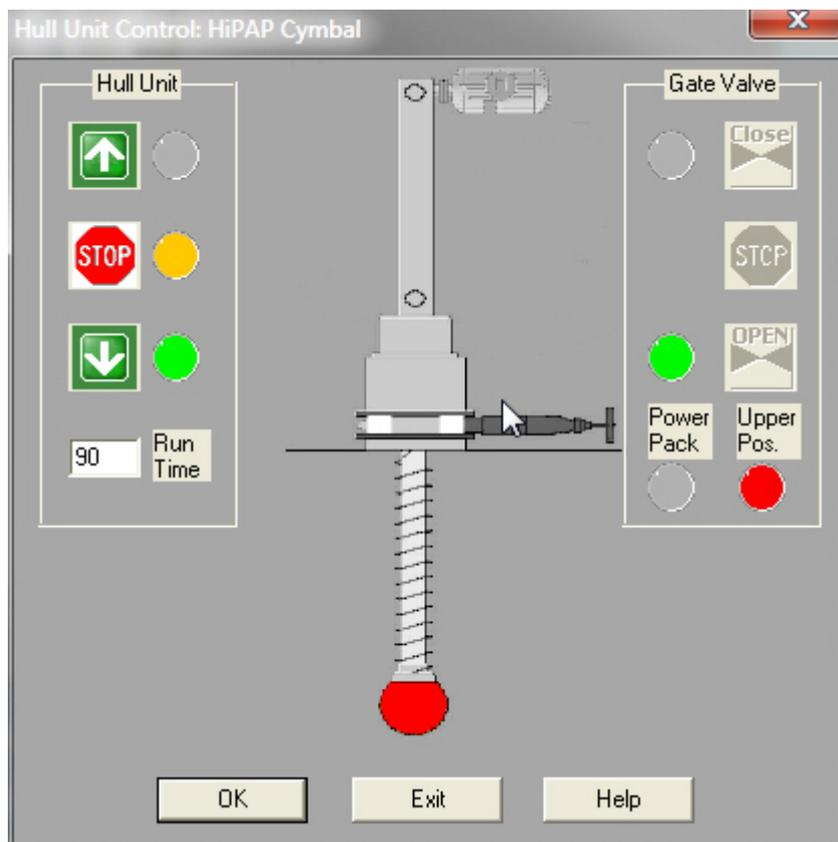
An alarm may be given if the hull unit is extracted and the vessel starts moving, see [Hull Unit Alarm](#)
