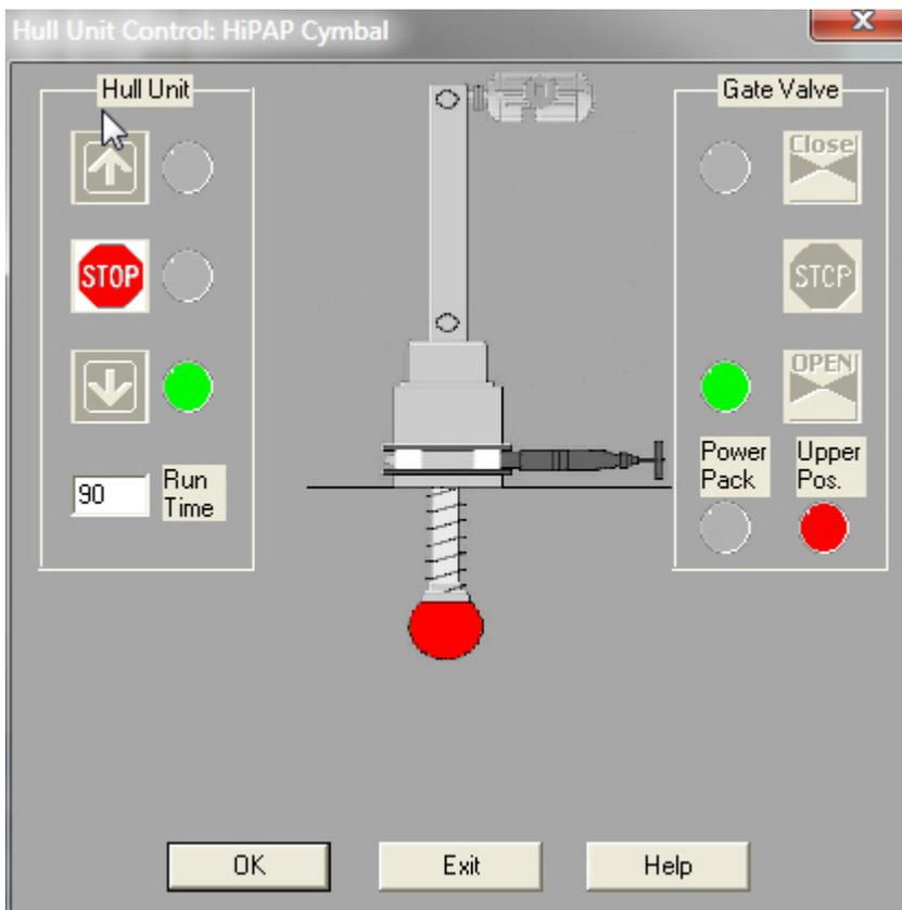
The indicator beside the down arrow will start flashing while the hull unit moves. The operation will take approximately 90 seconds for a standard hull unit. The hull unit in the middle will mimic the operation.
