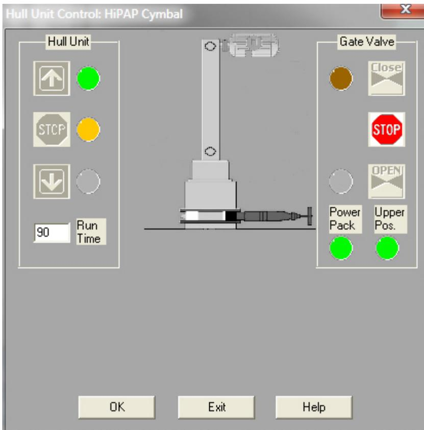
Pressing the Close button will start the operation and the accompanying indicator will start to flash yellow. The hull unit Gate Valve in the middle will mimic the operation.
