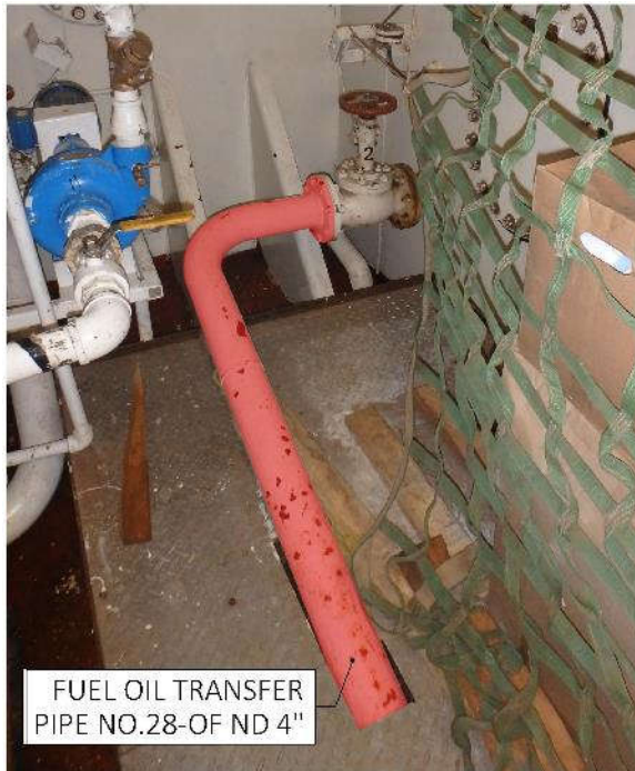
Figure 16 Fuel oil transfer, connection at bulkhead 146
