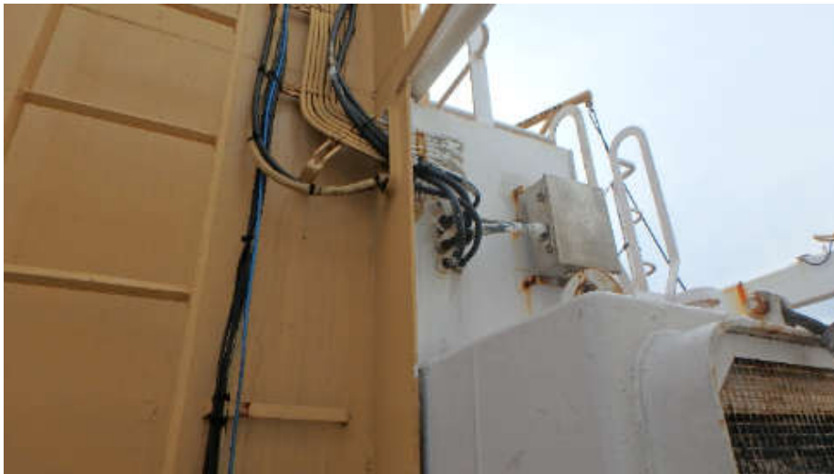
Figure 36 Existing cables between aft mast and emergency generator compartment
