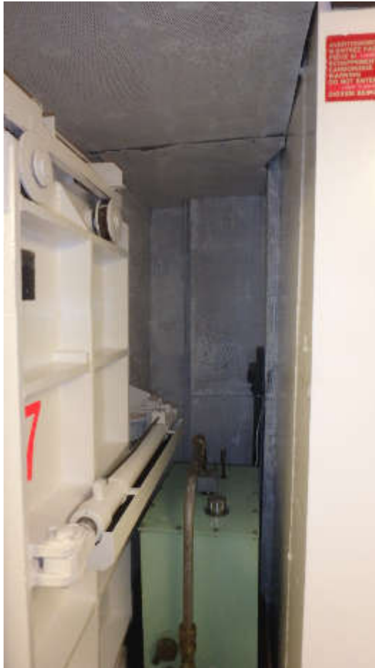
Figure 40 Watertight door recess, main deck starboard inboard, at frame 165. See bow thruster hydraulic oil header tank
