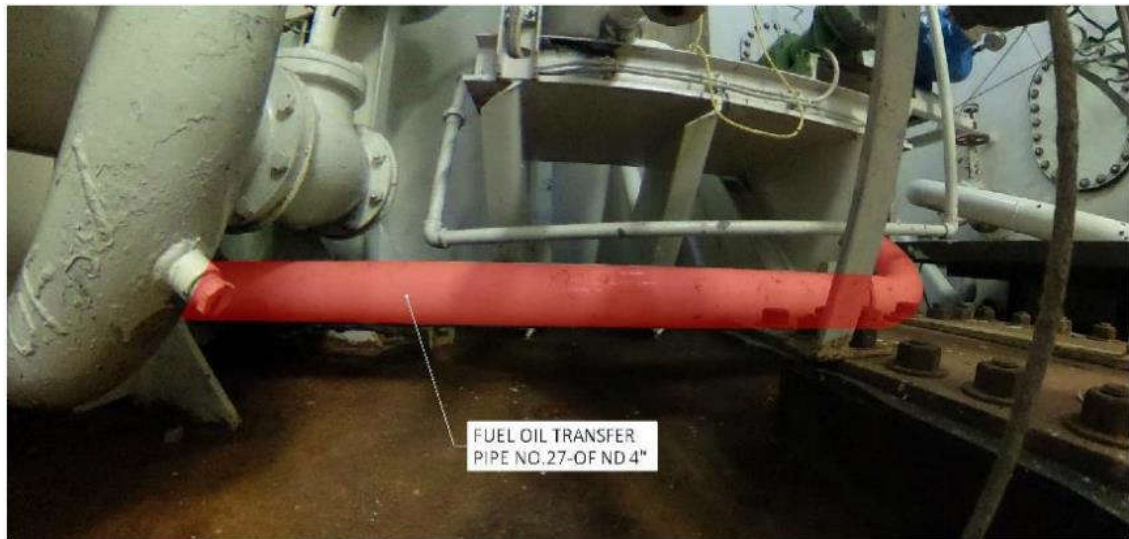
Figure 18 Fuel Oil transfer 27-OF, connection at bulkhead 138
