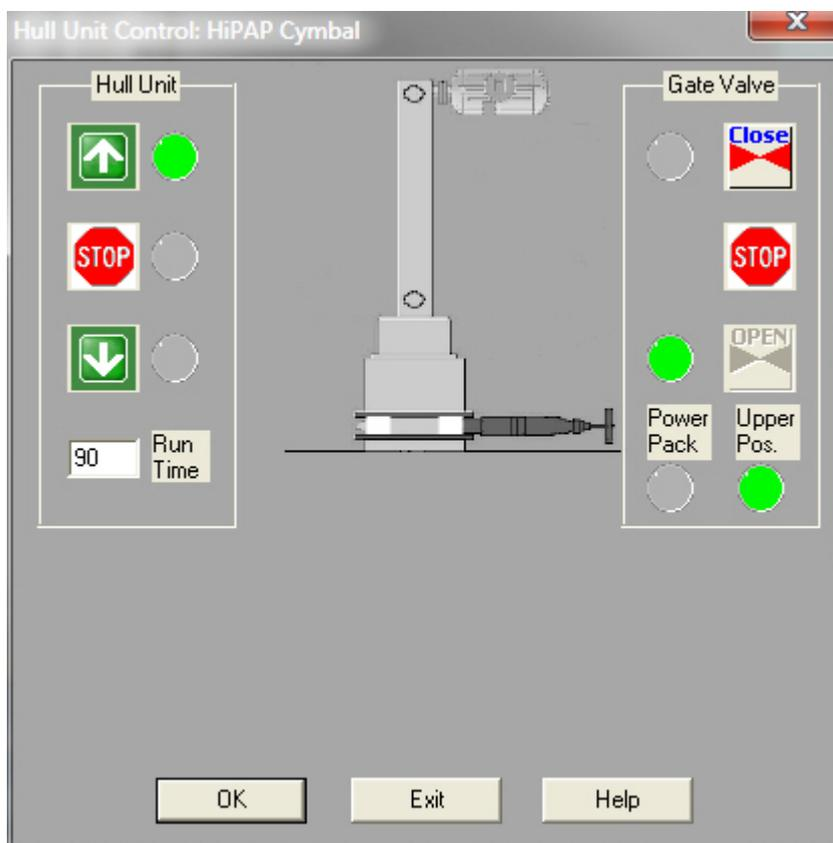
The dialog shows the hull unit in the upper position (left side of dialog) and the gate valve open.
