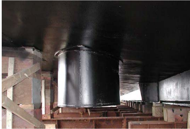
Figure 2. Blister drawing (top left), front of installation (top right) and rear (lower) view of the blister for the transducers. In this case the blister is located about 1 meter outboard of the keel.
