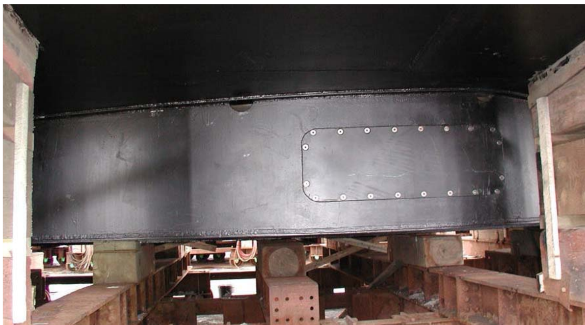
Figure 3. Side view of the blister showing the cable access plate (upper) and bottom view showing transducer placements (lower).
