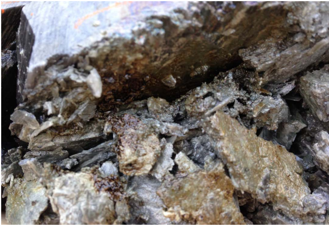
Photo 9: At location MW17-03, close up view of light non-aqueous phase liquid in fracture area at 7.6 m along the core axis (vertical projection of 5.4 mbgs). The bedrock at this location is limestone.
