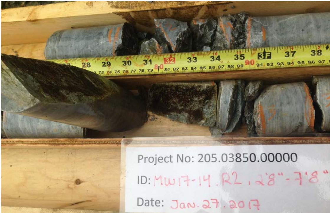
Photo 7: At location MW17-14, LNAPL observed in fractures at a depth of 1.4 m along the core axis (vertical projection of 1.0 mbgs). The bedrock at this location is limestone.
