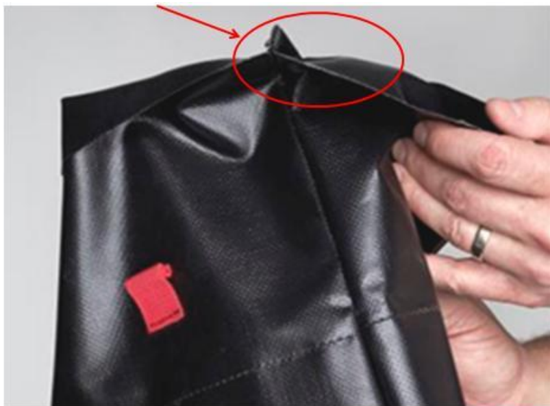
Picture no.01 Four ply seams (Outer Bag)
