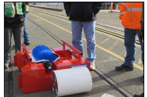
Spill response equipment: Skimmer.
