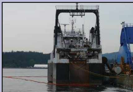
An orange inshore containment boom fully surrounds the vessel while being fuelled.
