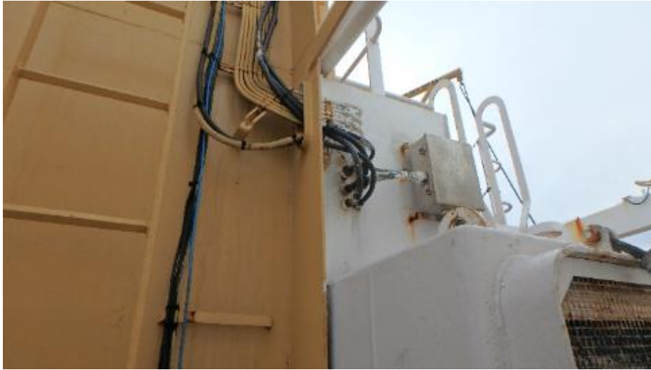
Figure 35 Existing cables between aft mast and emergency generator compartment
