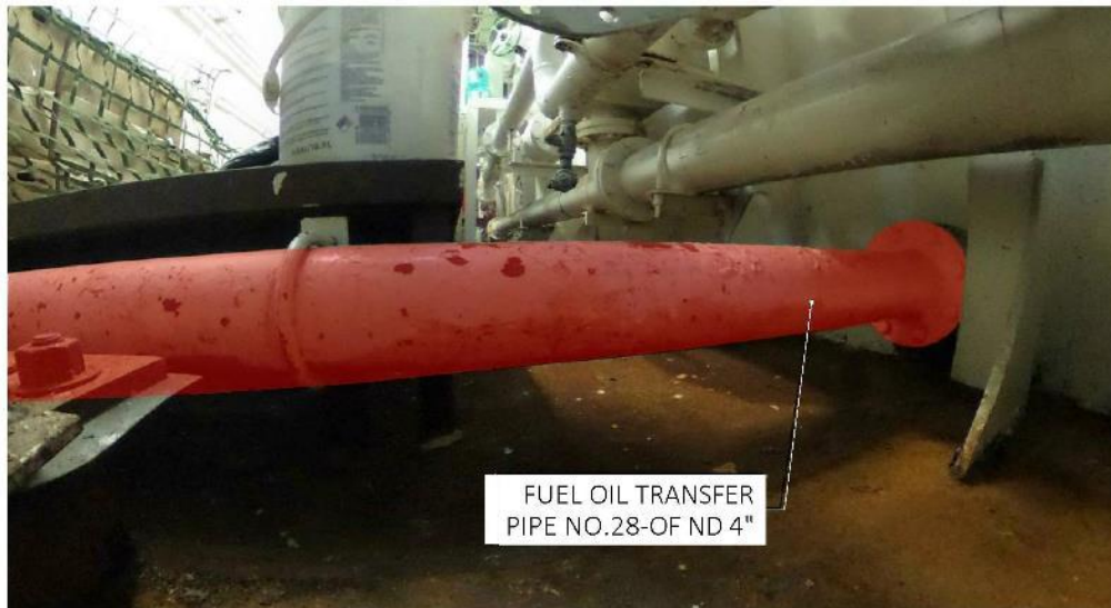
Figure 16 Fuel oil transfer, connection at bulkhead 138
