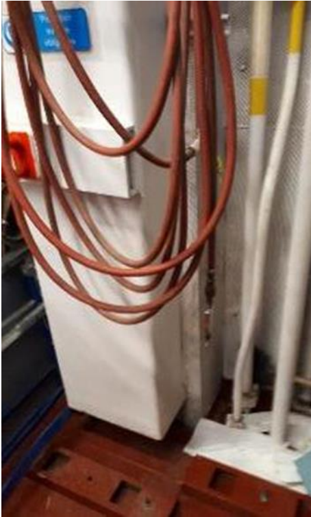
Figure 32 Existing cargo hold air outlet to be modified
