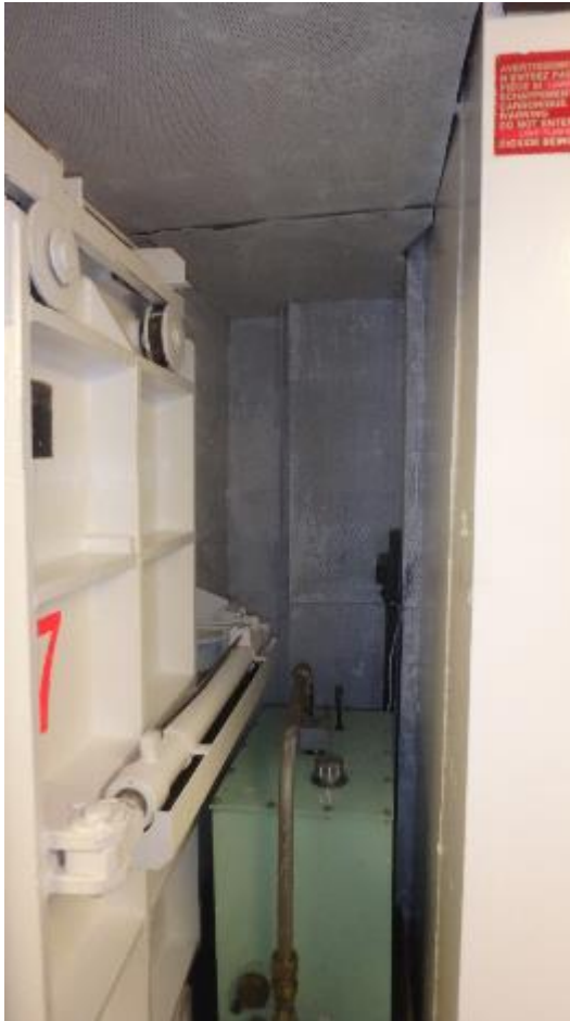
Figure 39 Watertight door recess, main deck starboard inboard, at frame 165. See bow thruster hydraulic oil header tank
