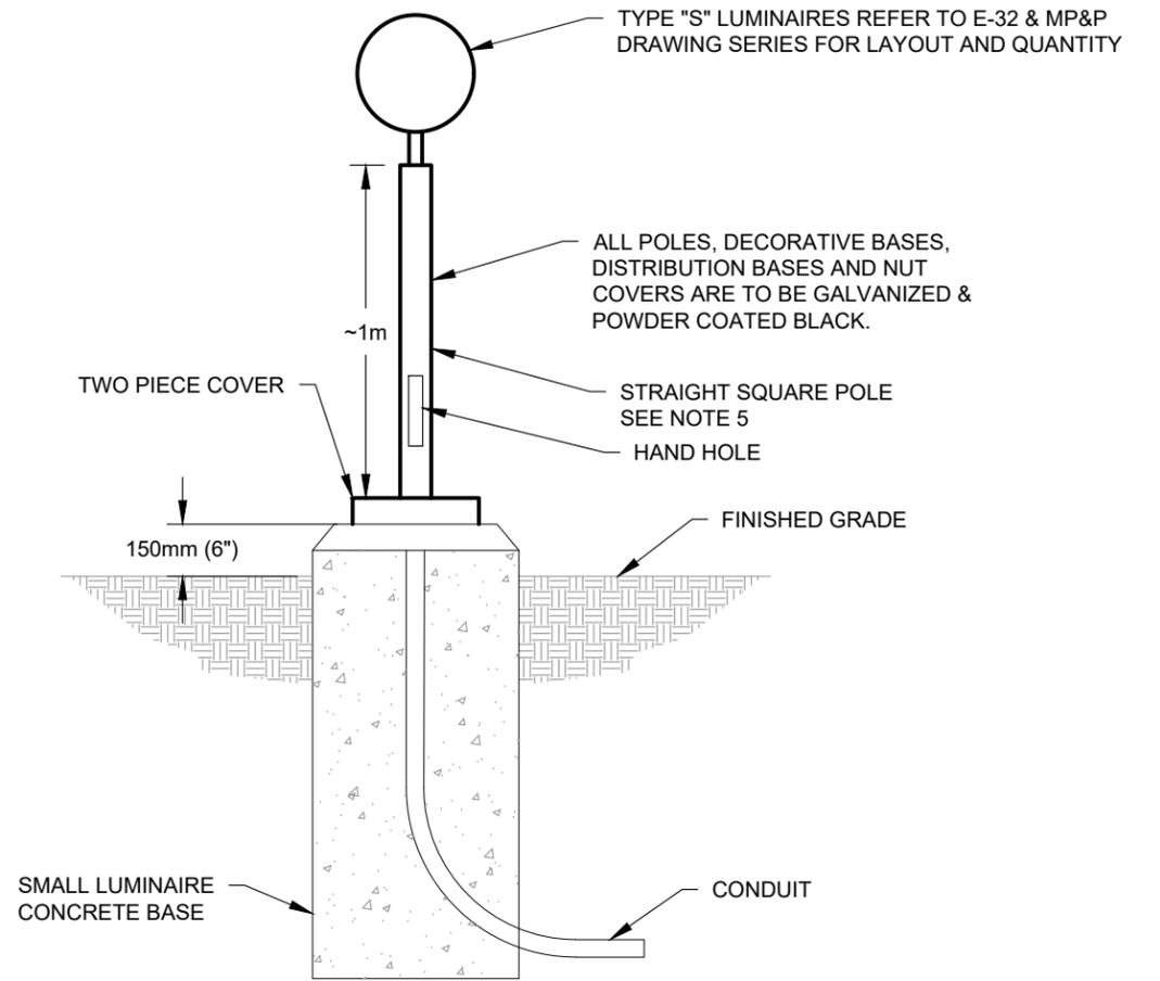
**DETAIL 8 - POLE LUMINAIRE FIXTURE TYPE "S1"**
