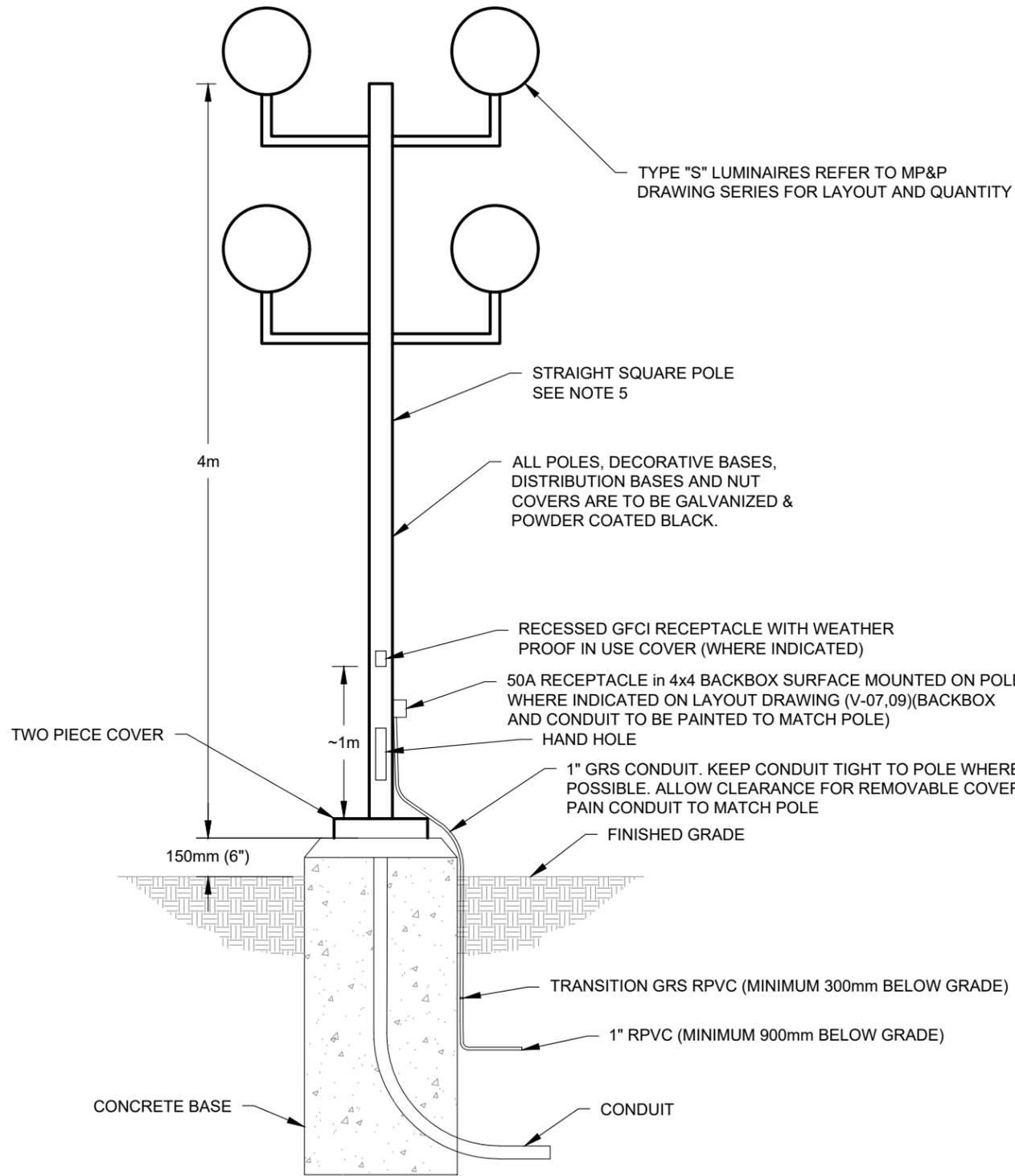
**DETAIL 3 - POLE LUMINAIRE FIXTURE TYPE "S"**
