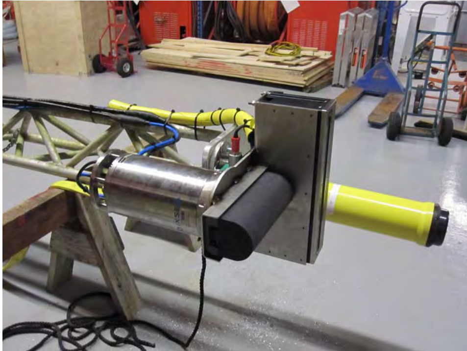
Figure 20: Custom fabricated sensor frame
