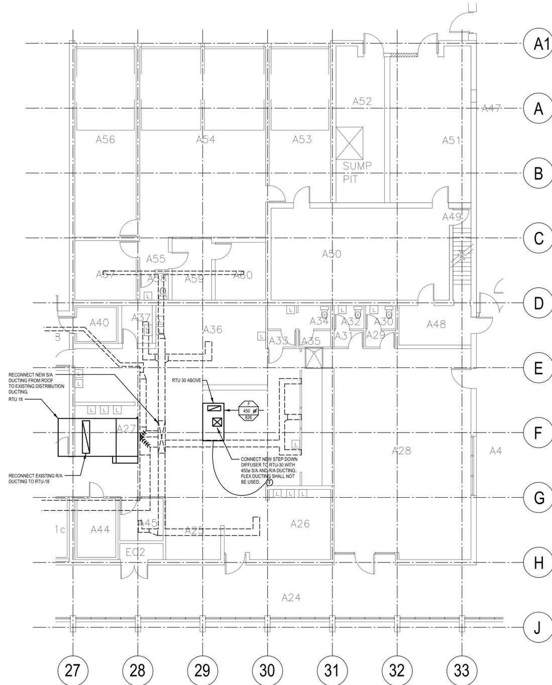
GENERAL NOTES: 1. CONFIRM LOCATION OF RTU 30 PRIOR TO ANY CUTTING OF ROOF. UNIT SHALL BE PLACED GENERALLY AS SHOWN, BUT CAN BE ADJUSTED SLIGHTLY TO AVOID CLASHES IN THE KITCHEN CEILING SPACE. DO NOT CUT STRUCTURE.
