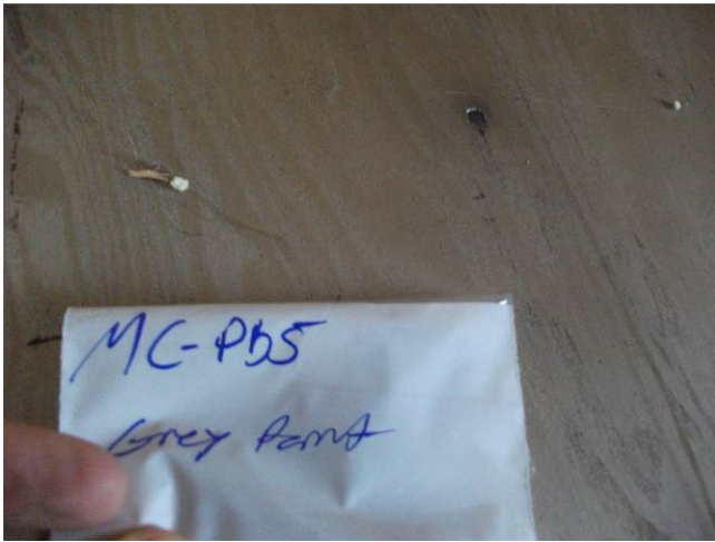
Photograph 13: Metal Clad Storage Building – Lead-Based Grey Wall Paint
