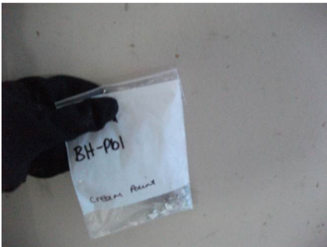
Photograph 27: Boat House Building – Lead-Based Cream Wall Paint
