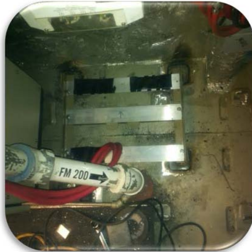
Figure 10 New position of battery mounting bracket
