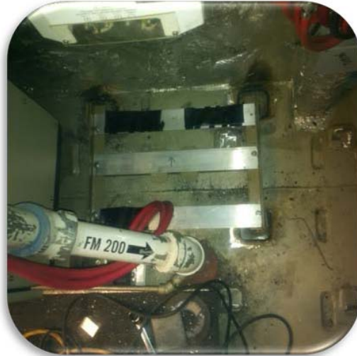
Figure 10 New position of battery mounting bracket
