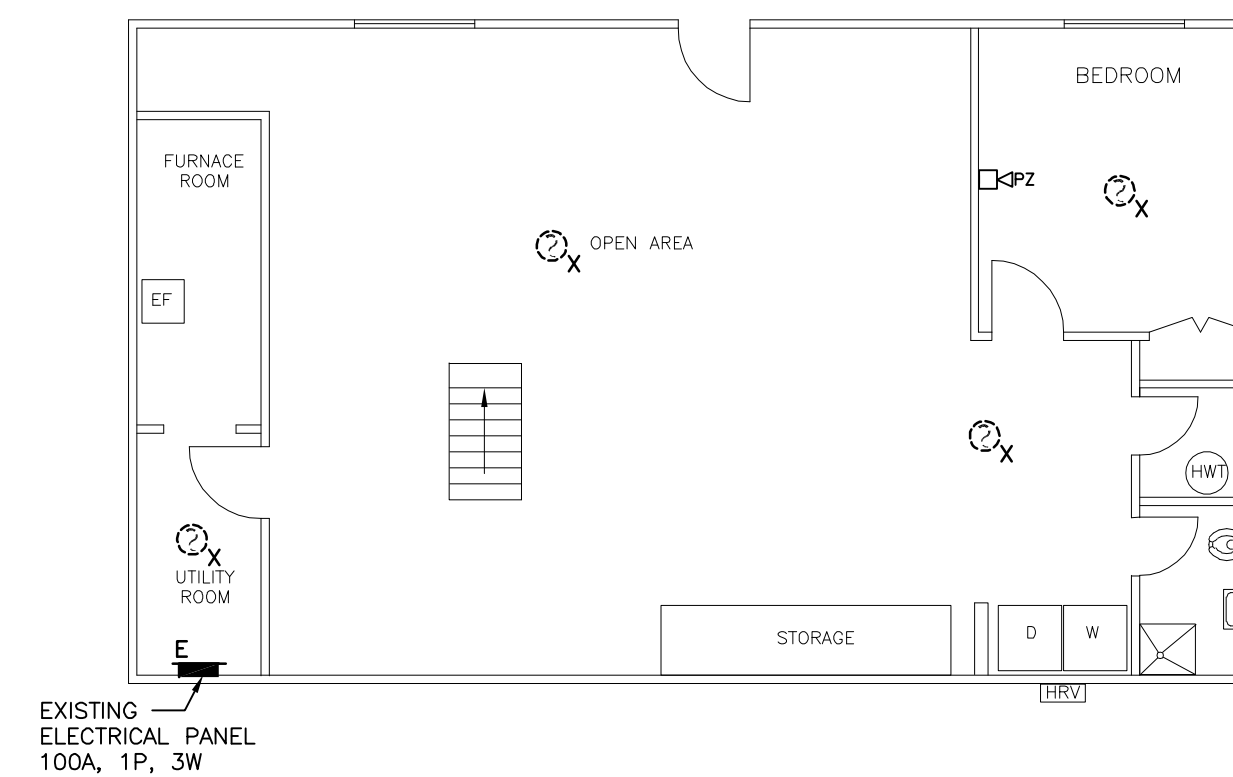
3 UNIT 7-BASEMENT-DEMOLITION-FIRE ALARM SYSTEM E-4 SCALE: 1/8"=1'-0"
