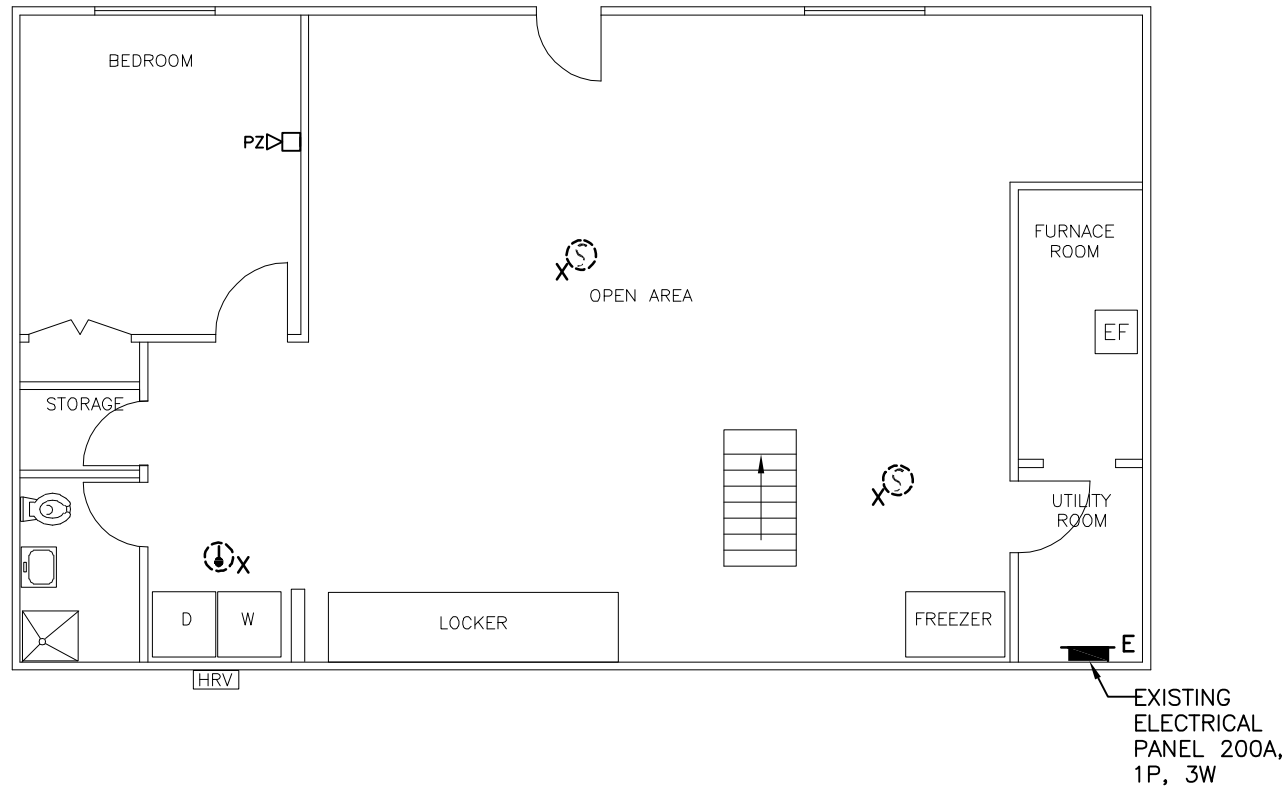
1 UNIT 4-BASEMENT-DEMOLITION-FIRE ALARM SYSTEM E-3 SCALE: 1/8"=1'-0"
