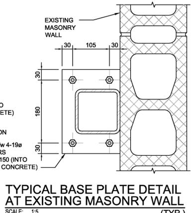
**TYPICAL BASE PLATE DETAIL AT EXISTING MASONRY WALL**
