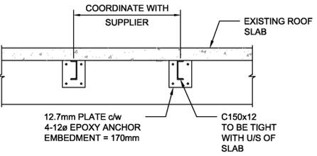
**J SECTION - CONSTRUCTION DETAIL**
