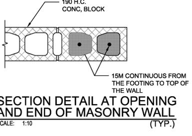
**SECTION DETAIL AT OPENING AND END OF MASONRY WALL**
