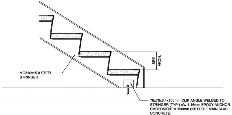
**L DETAIL - STAIR CONNECTION AT LEVEL 2**
