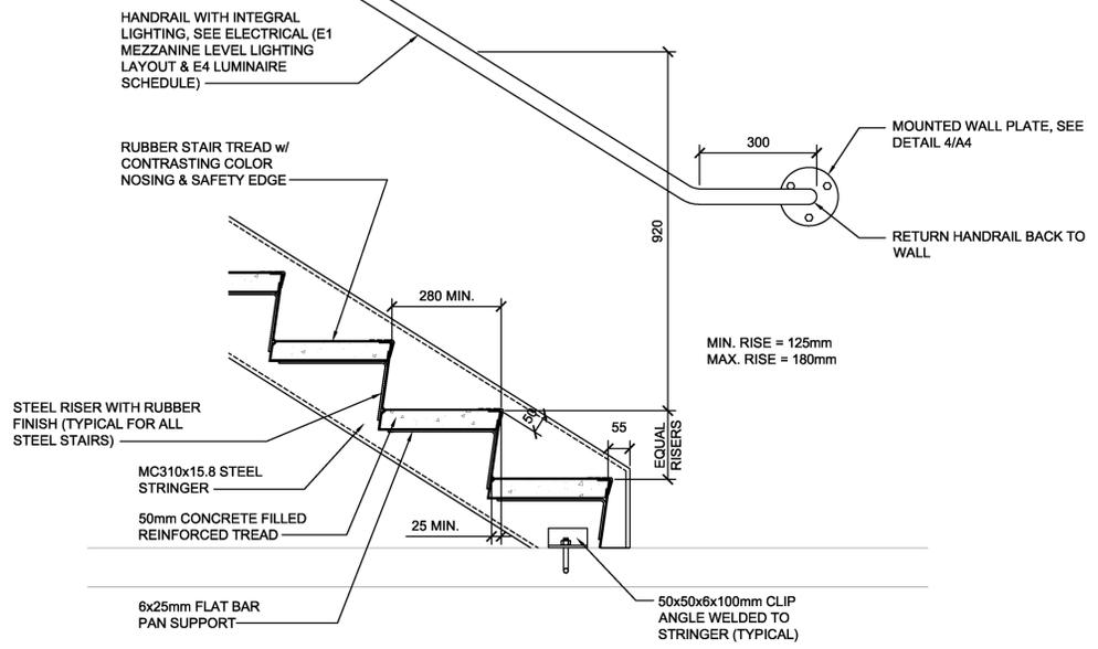
DETAIL - STAIR AND WALL ATTACHED HANDRAIL 5
