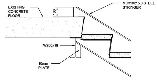
**K DETAIL - STAIR CONNECTION AT MEZZANINE FLOOR**
