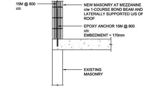
**H SECTION - CONSTRUCTION DETAIL**
