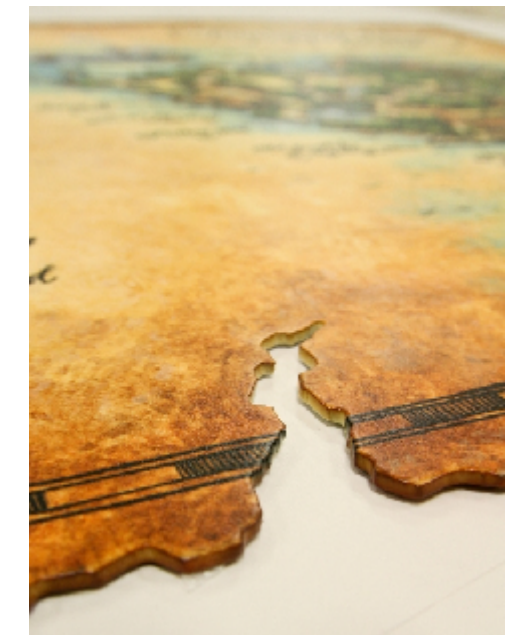
TYPICAL EDGE TREATMENT - ROUTERED PANEL
