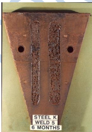
Figure 15 - Weld Metal Corrosion
