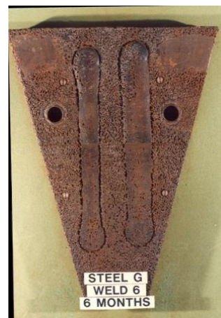
Figure 16 - HAZ Corrosion
