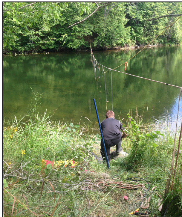
Figure 4: River Crossing Seismic Line with Geophones & Hydrophones
