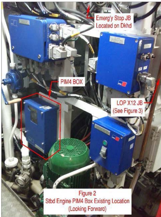
Figure 2: Stbd Engine PIM 4 Box existing location looking fwd
