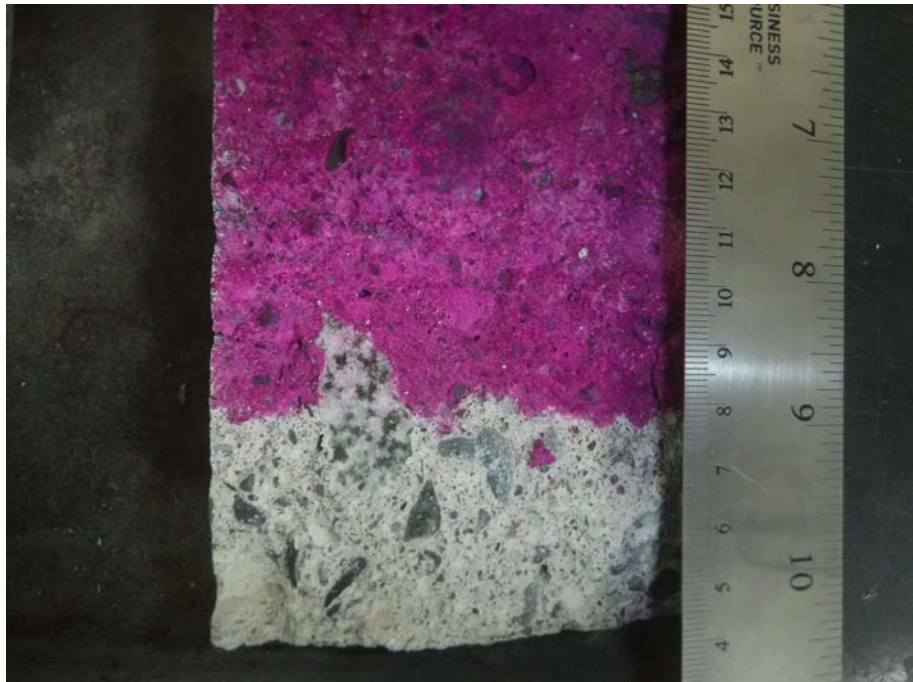
Photo 2: Core sample fractured surface treated with phenolphthalein
