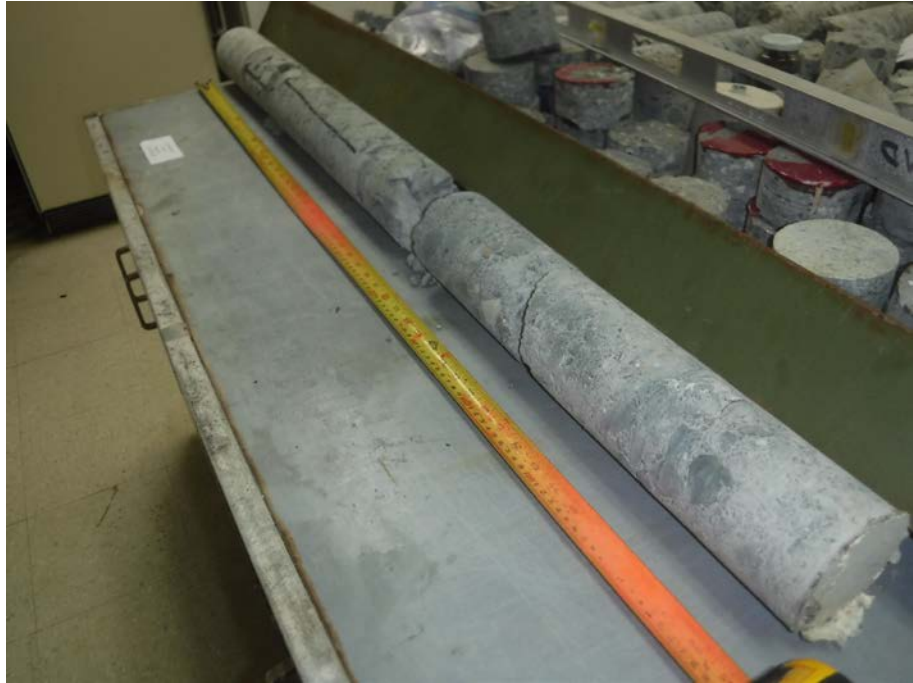
Photo 5: Full-thickness core from "magazine" roof slab
