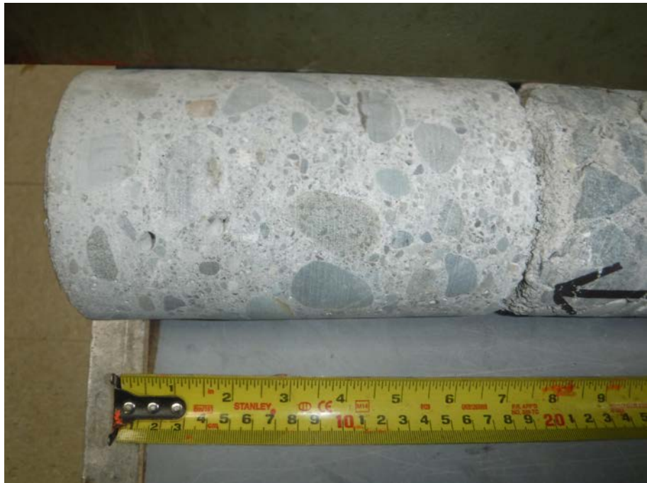
Photo 6: Concrete topping at the top end of full-thickness core
