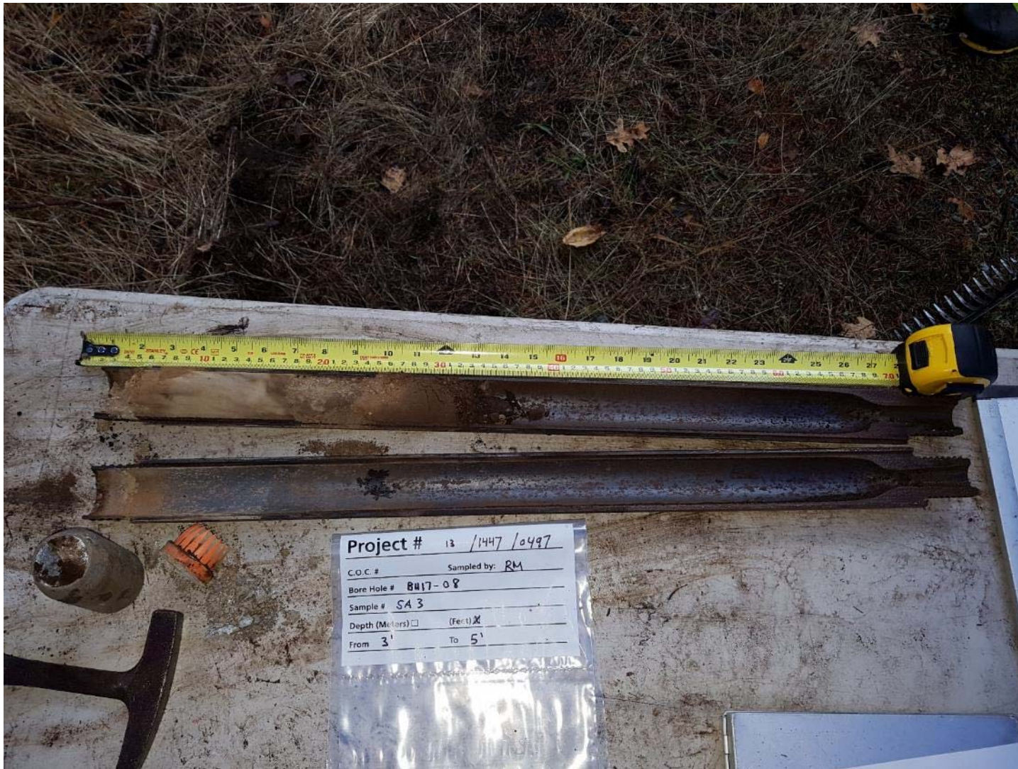
Photograph 12: Example of a Standard Penetration Test (SPT) – Split Spoon Sample at the north Searchlight Engine Room Retaining Wall (BH17-08)
