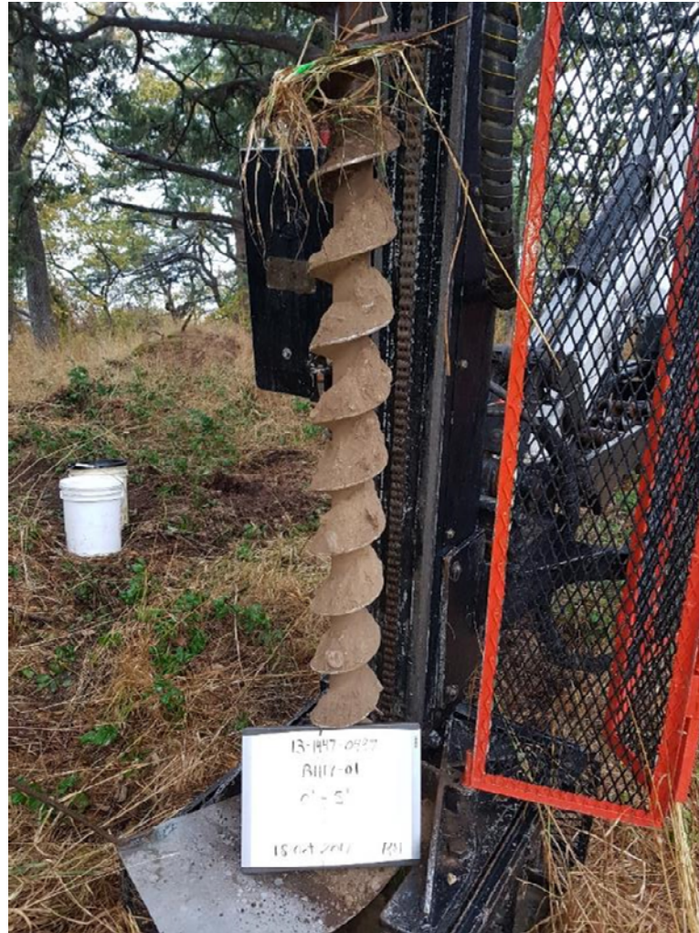
Photograph 14: Example of silt to silty sand fill material at the Searchlight Engine Room (BH17-01)
