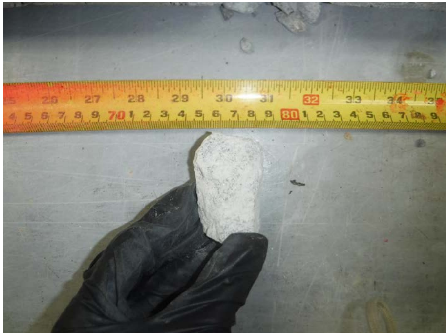
Photo 12: Coarse aggregate from full-thickness core
