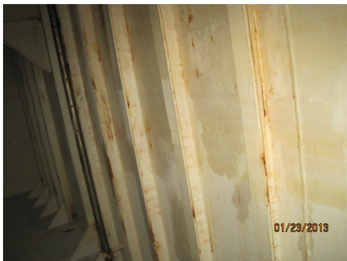
4.83: Fresh Water Tank Starboard - Longitudinal Bhd
