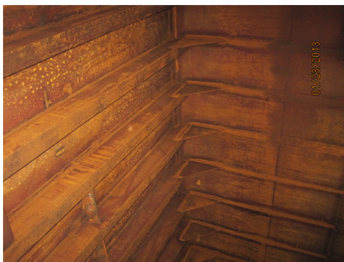
4.34: F.O. Deep Tank Port - Longitudinal Bhd & Deck
