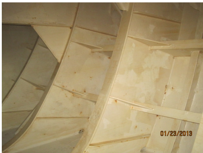
4.81: Fresh Water Tank Port - Side Shell
