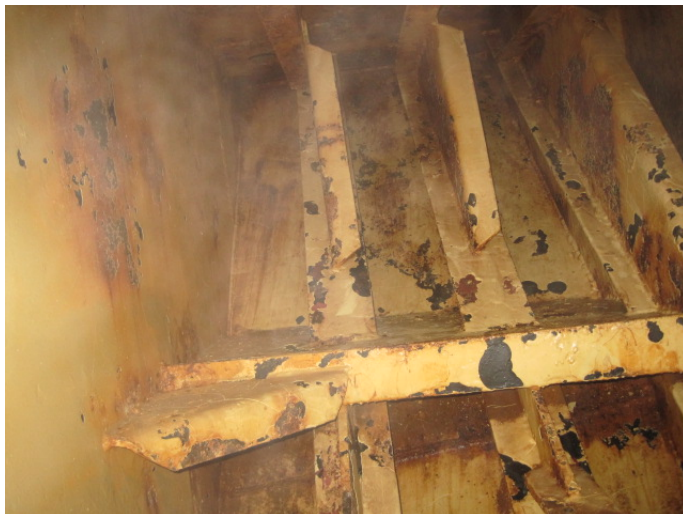
4.19: FPT Under Chain Locker - Side Shell
