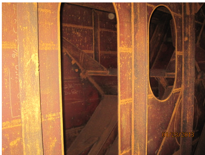
4.33: F.O. Deep Tank Port - Structure
