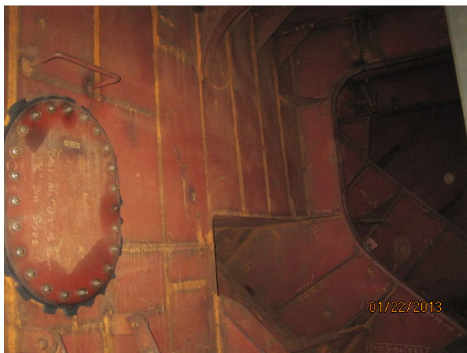
4.43: Fwd F.O. Tank Port - Longitudinal Bhd & Structure
