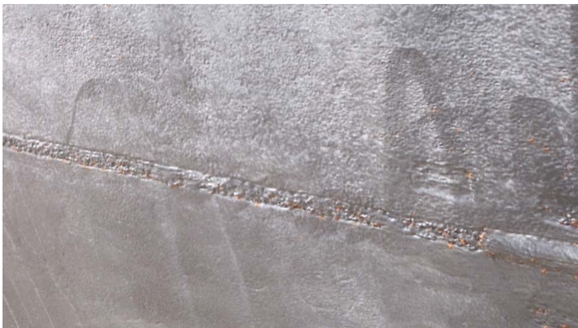
4.3: Port Side Hull Fwd Half – Eroded Weld
