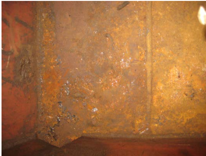
4.42: Fwd Engine Room Wing Tank Starboard - Typical Corrosion At Lower Level
