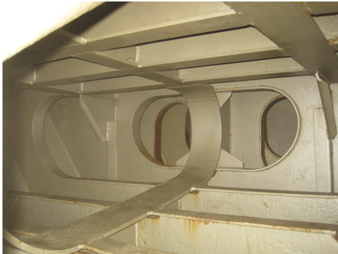
4.108: No.5 Void Space – Internal Structure
