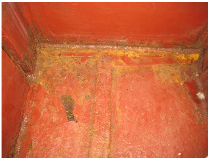
4.104: Fwd DP Thruster Cofferdam - Bottom Mild Corrosion
