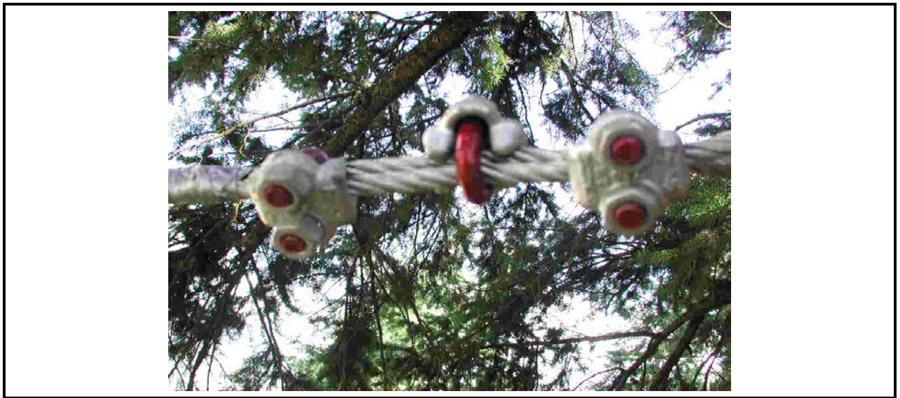
Figure 11A-3 Placement of Bolt Connectors Onto Safety Cables
