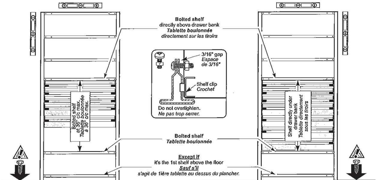
Shelving unit must be anchored to the floor or to the wall structure.
