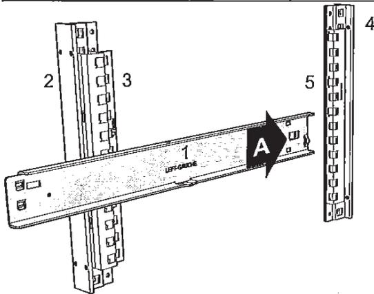
**A** Insert the rear hook of the rail into the rectangular slot of the rear mounting bracket.
