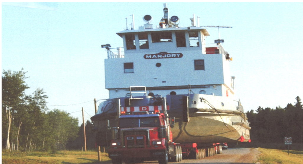
MV "Marjory" on Slave River Rapids Portage, carried by Mammoet Canada's Heavy Haul Trailers
