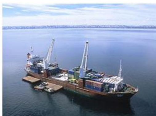
MV Umiavut offloading cargo to lighter barges for delivery to a sealift beach. Nunatsiqa News Photo
