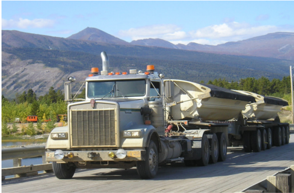
Crossing Nares River Bridge at Carcross, Yukon, Canadian Lynden Transport bulk haul permitted "Super B" train carrying 53 tonnes of copper concentrate from Minto Mine to the Skagway, Alaska ore terminal.
