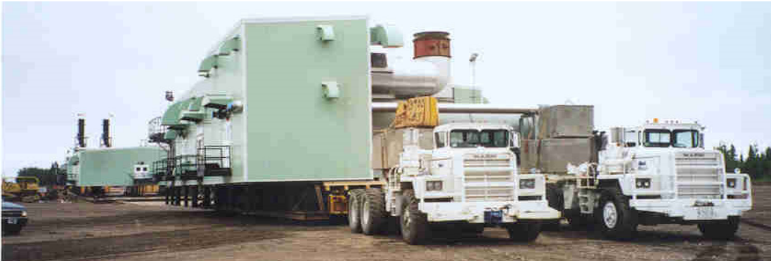
Badami Oil Field Modules Transferring from Road to Barge at Hay River, N.W.T.
