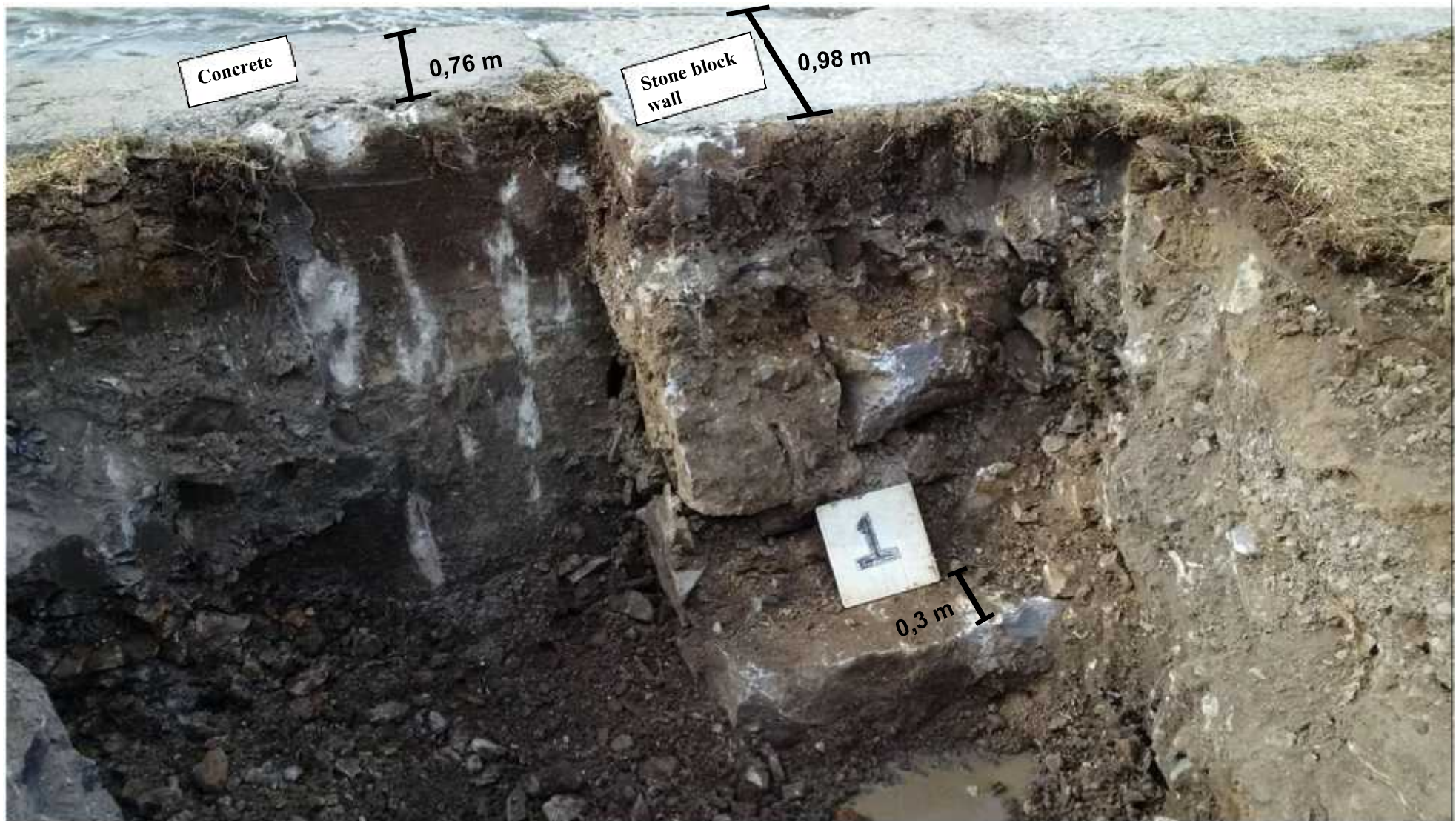
Photo 1 – Test pit TR-01 – Concrete and stone block wall junction
