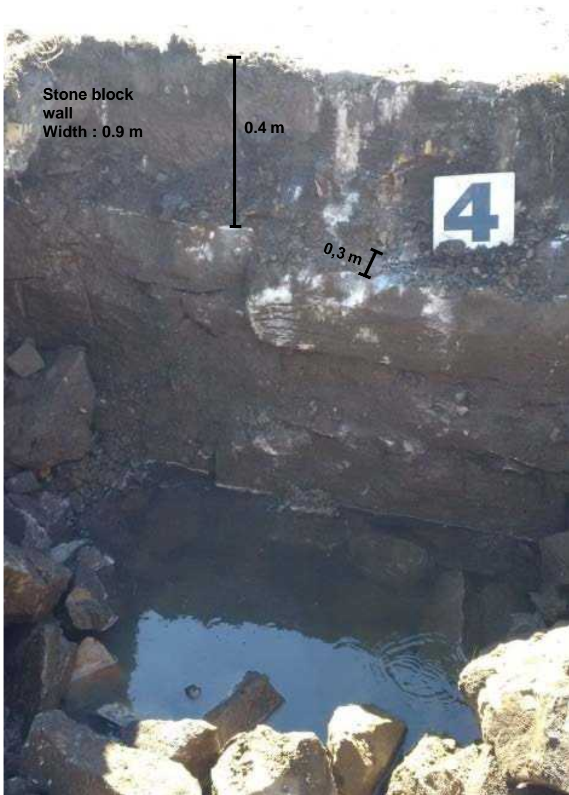
Photo 4 – Test pit TR-04 – Stone block wall
