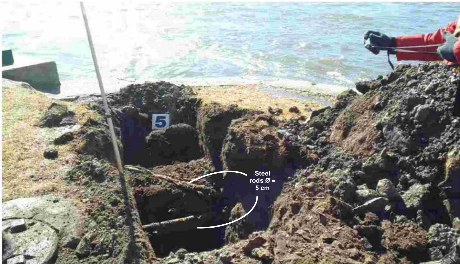
Photo 5 – Test pit TR-05 – Concrete wall with steel rods
