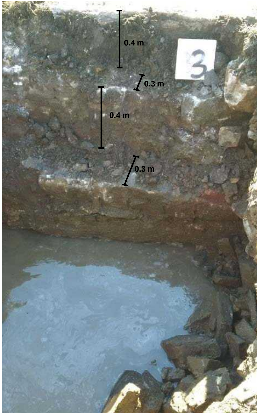
Photo 3 – Test pit TR-03 – Stone block wall
