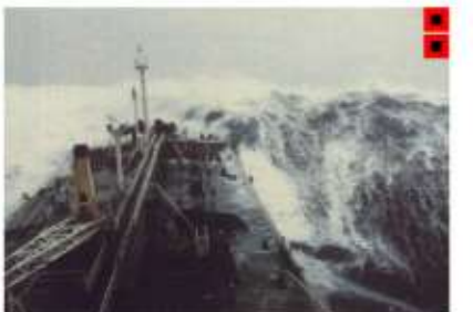
BEAUFORT FORCE 11 WIND SPEED: 64 KNOTS SEA: SEA COMPLETELY WHITE WITH DRIVING SPRAY, VISIBILITY VERY SERIOUSLY AFFECTED, THE AIR IS FILLED WITH FOAM AND SPRAY
