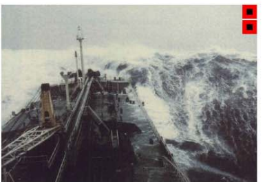
BEAUFORT FORCE 12 WIND SPEED: 64 KNOTS SEA: SEA COMPLETELY WHITE WITH DRIVING SPRAY, VISIBILITY VERY SERIOUSLY AFFECTED, THE AIR IS FILLED WITH FOAM AND SPRAY
