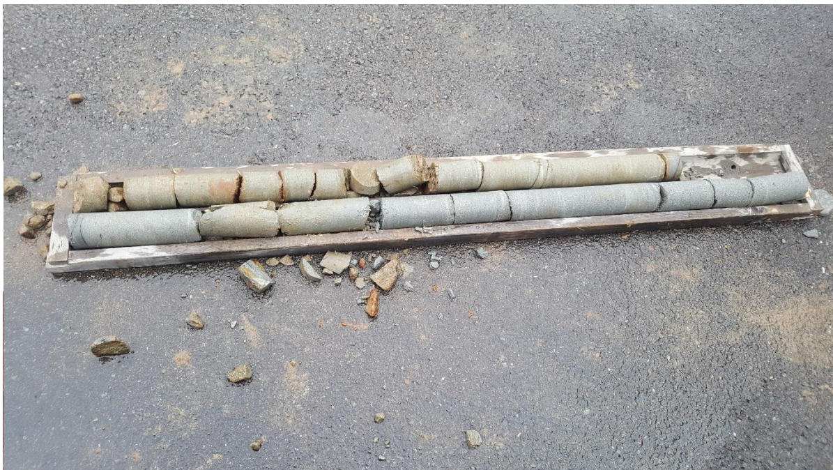
Photo 8: BH-04 / Rock Cores
