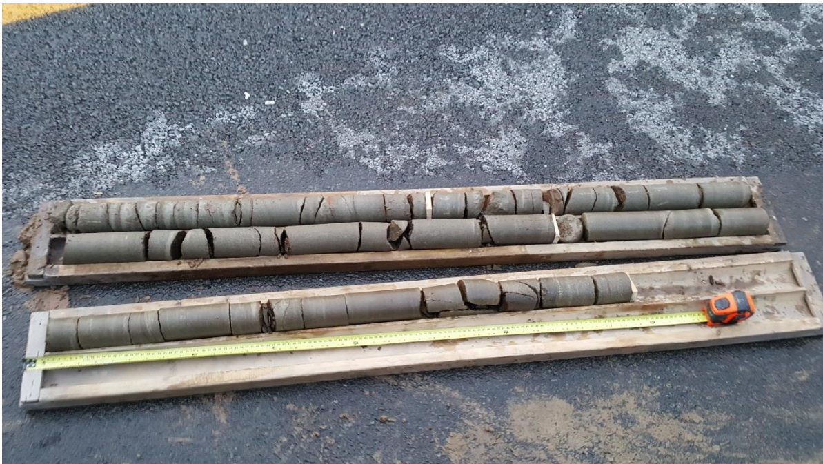
Photo 6: BH-02 / Rock Cores
