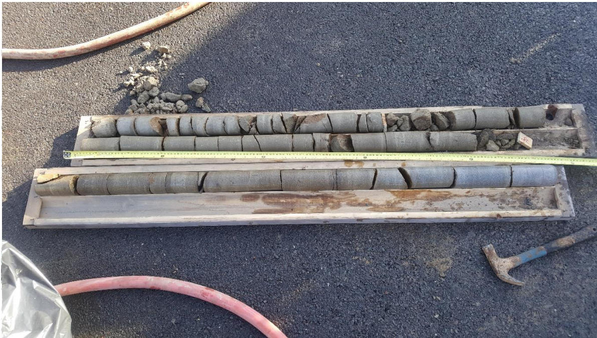
Photo 7: BH-03 / Rock Cores
