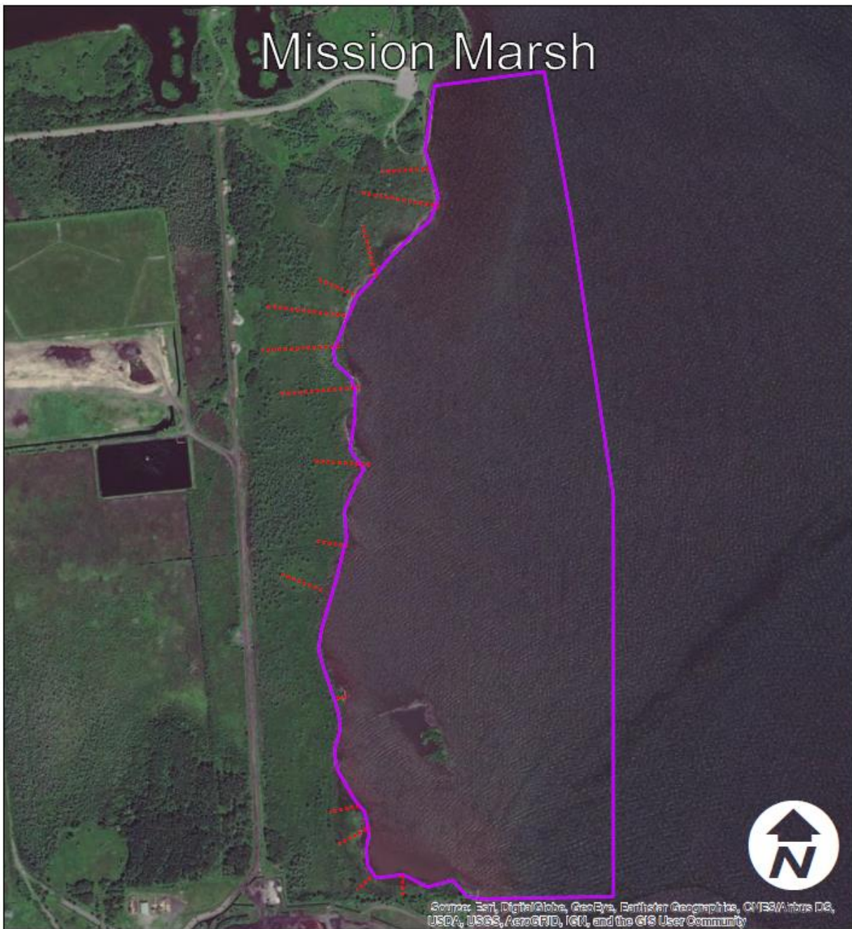
Figure 11. Map illustrating the locations of topographic survey transects and general bathymetric survey extent for Mission Marsh.
