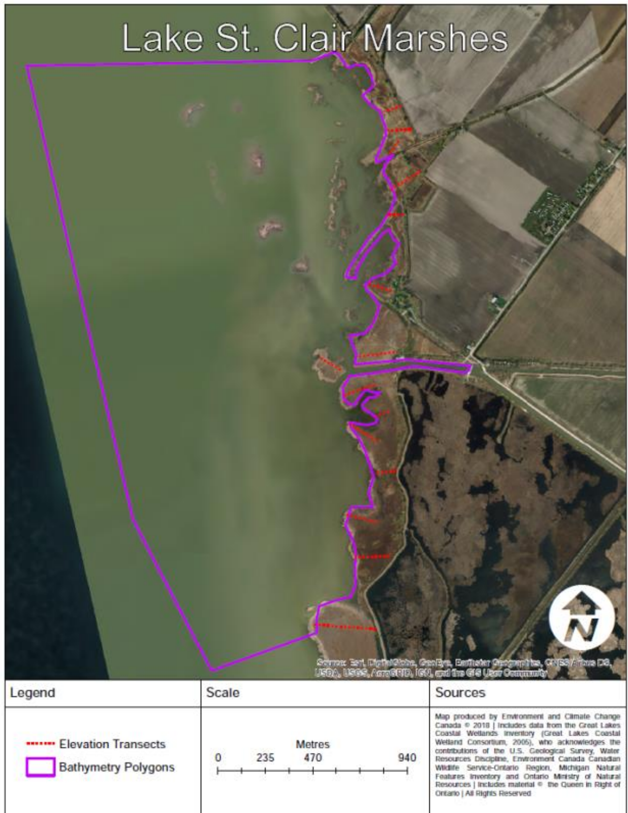
Figure 13. Map illustrating the locations of topographic survey transects and general bathymetric survey extent for Lake St. Clair Marshes
