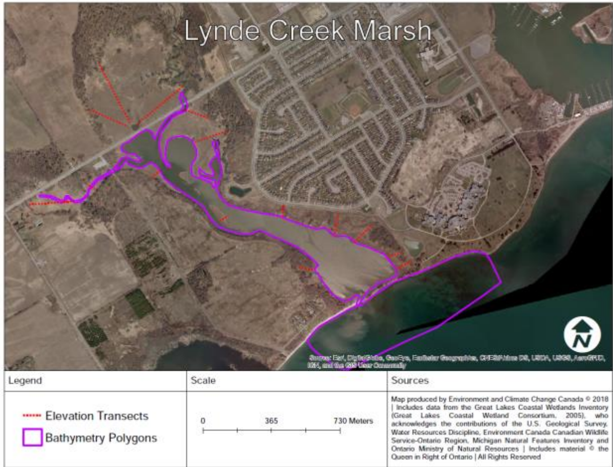
Figure 5. Map illustrating the locations of topographic survey transects and general bathymetric survey extent for Lynde Creek Marsh.
