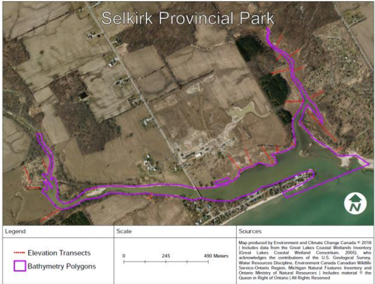
Figure 11. Map illustrating the locations of topographic survey transects and general bathymetric survey extent for Selkirk Provincial Park.
