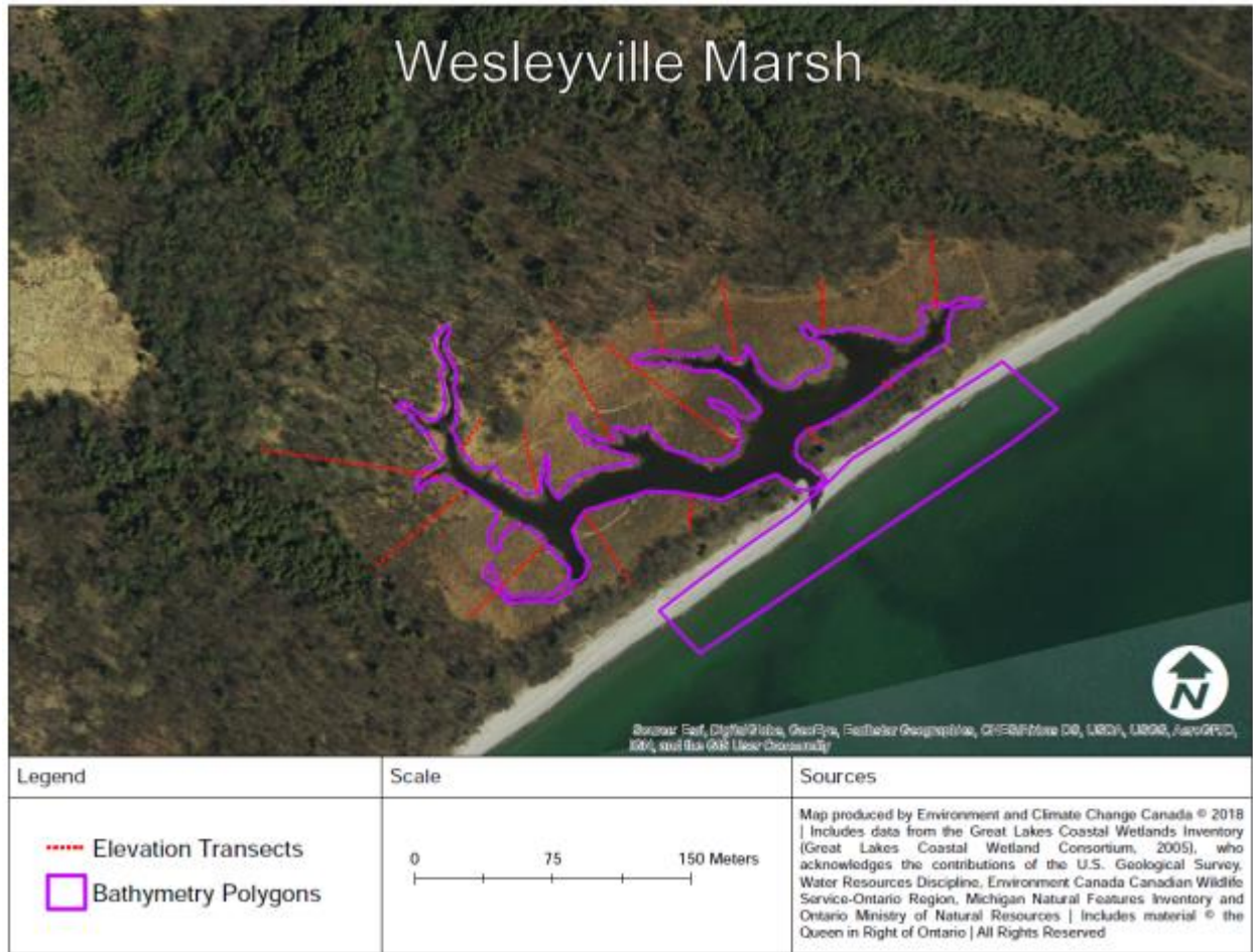
Figure 7. Map illustrating the locations of topographic survey transects and general bathymetric survey extent for Wesleyville
