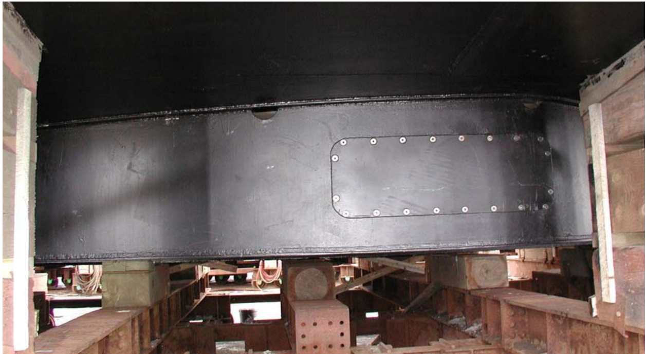
Photo 5. View of the blister's base and transducers, looking forward.
