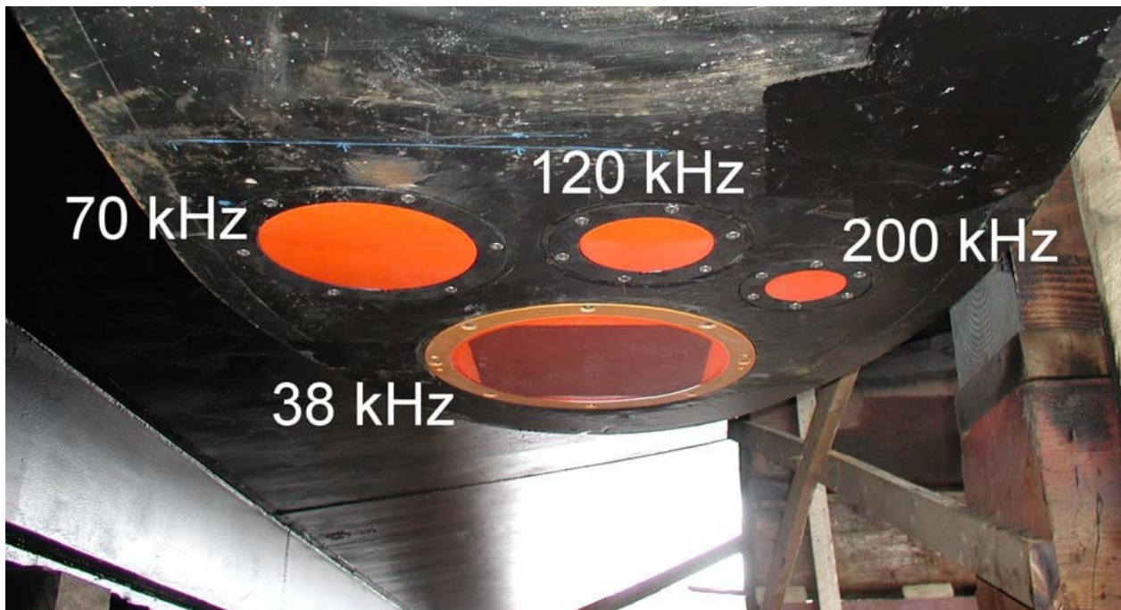
Photo 5. View of the blister's base and transducers, looking forward.
