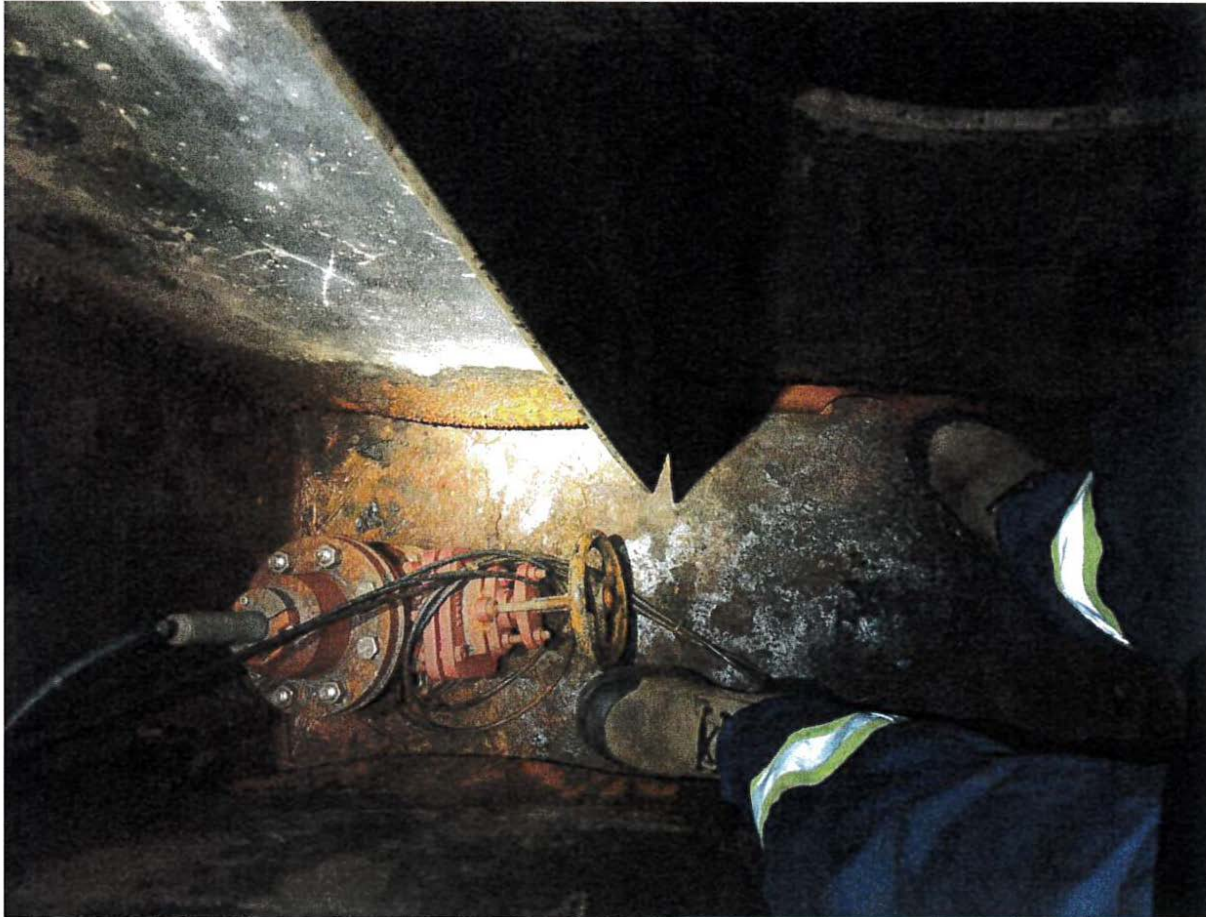
Photograph 8 – View of transverse floor plate in transducer compartment. Buckling of lower edge of floor plate consistent at each frame in way of damage.
