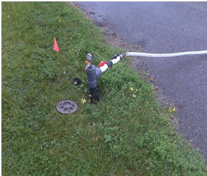
Picture 1: Attachment injection fixture at monitoring wells
