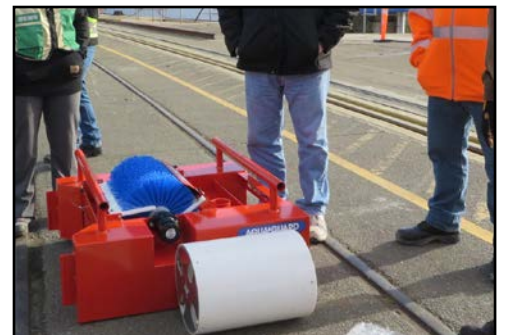
Spill response equipment: Skimmer.
