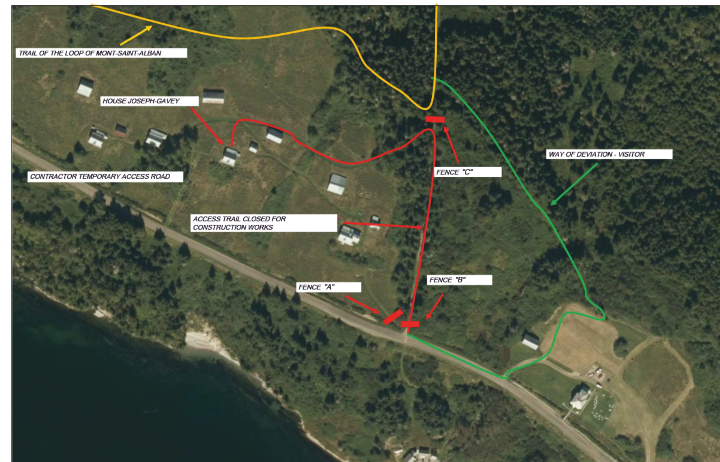
TEMPORARY SIGNALING FOR THE DURATION OF WORK WITH THE EXCEPTION OF THE PERIOD SEPTEMBER 21 TO 23, 2018 FENCES "A", "B", "C" SHOWING : "CONSTRUCTION SITE. NO PUBLIC ACCESS"
