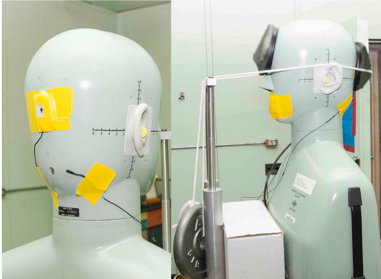
Figure C-4: Headset TTC and Noise Reduction Test Setup (1/2)
