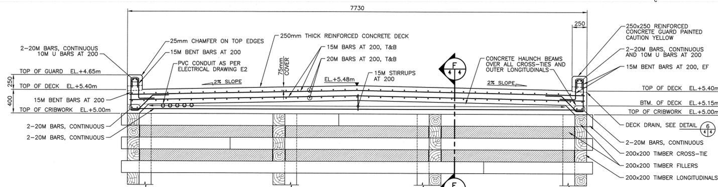
TYPICAL WHARF CONCRETE DECK ON CRIBWORK BLOCK DETAIL (1/4)
