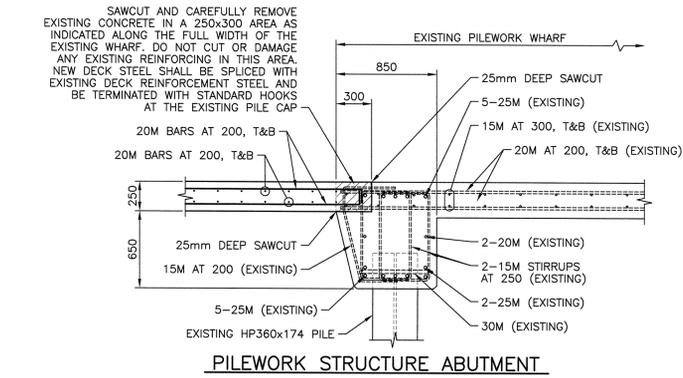
PILEWORK STRUCTURE ABUTMENT (F/4)
