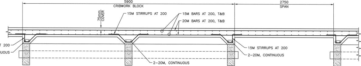
TYPICAL CRIBWORK BLOCK AND SPAN (2/4)
