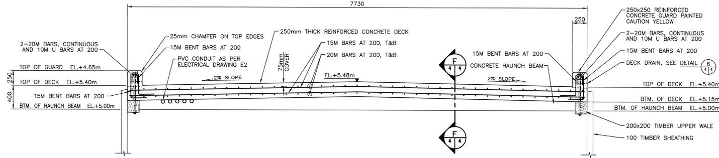
TYPICAL WHARF CONCRETE DECK ON CRIBWORK BLOCK DETAIL (2/4)
