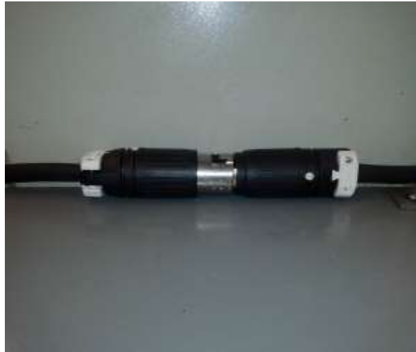
Figure 3-4 Electrical Power Plug used with an existing CNC Milling Machine
