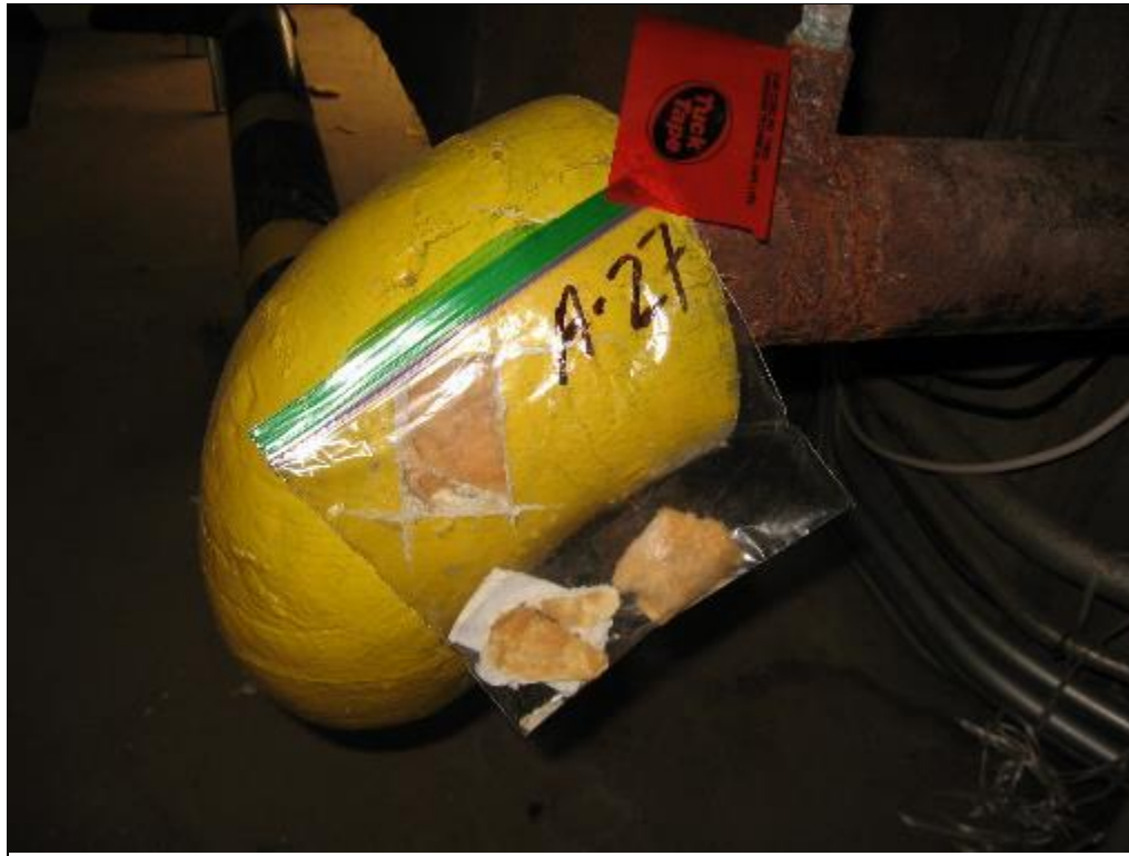
Photo 7: Insulating pipe cement (Sample No. A-27: 15 % Chrysotile asbestos) over fibreglass on 90 mm dia. elbow in Upper Mechanical Room. (8 Sept. 2016)
