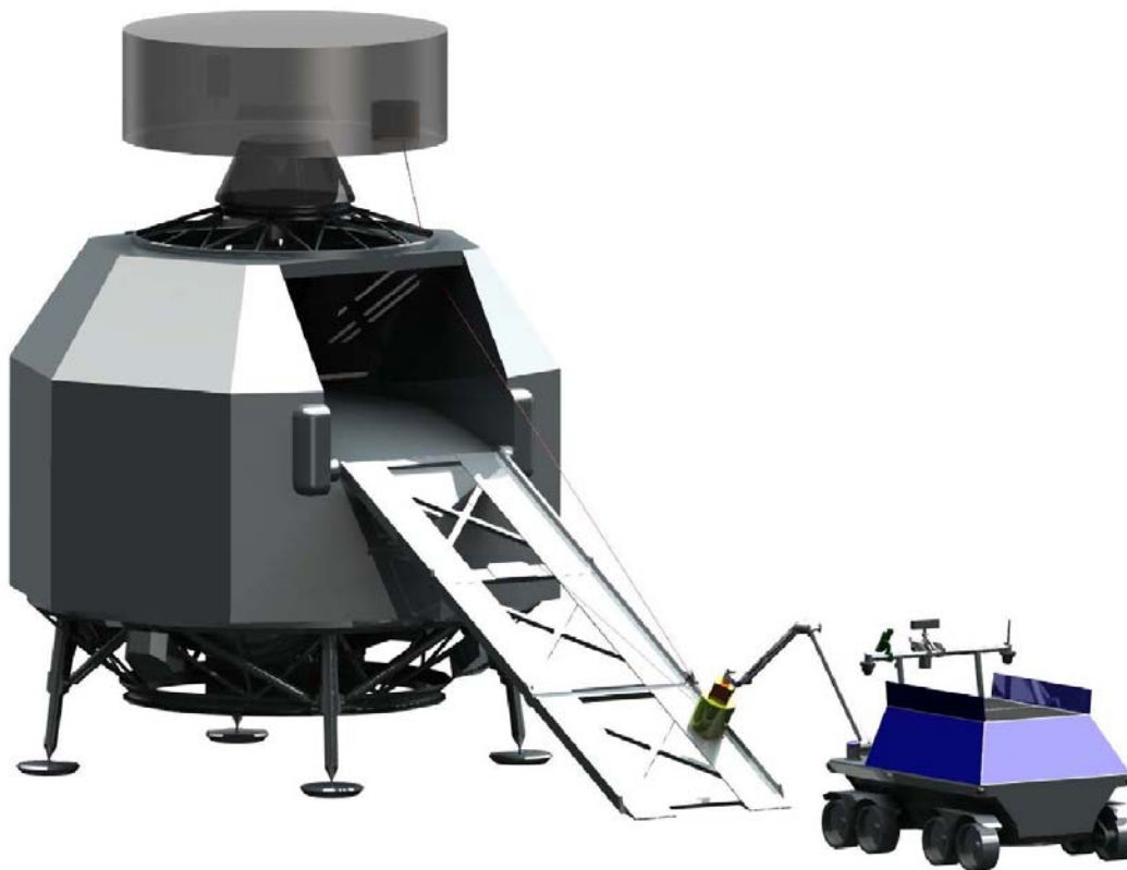
FIGURE 1-18: PHASR TRANSFERRING THE SAMPLE CONTAINER TO THE LANDER
