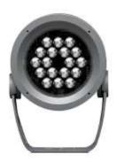
ROUND FLOOD FIXTURE, WALL MOUNT WITH HIGH-PERFORMANCE, LED FLOOD / ACCENT LIGHT AND LINEAR SPREAD LENS C/W DIMMING, DMX/RDM CONTROL CAPABILITIES AND BRACKET ARMS AND SELF CONTAINED TYPE, WHITE POWDER COAT FINISH. MODEL: LUMENBEAM #LBM-120-BLUE-NF-LSL-NO OR APPROVED EQUIVALENT. VOLTAGE: 120-277V DRIVER: DIMMABLE, BLUE COLOUR OUTPUT LAMP: 28W LED RGB (80 CRI)
