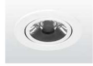
75 mm DIAMETER ROUND TRIM, RECESSED MOUNTED HIGH PERFORMANCE LED DOWNLIGHT WITH TILT CAPABILITY FOR BEAM ANGLES AND CLEAR GLASS LENS. 1000 NOMINAL LUMENS, MEDIUM ANGLE DISTRIBUTION AND IP54 RATING SUITABLE FOR WET LOCATION. NON-INSULATED INSTALL TYPE, WHITE POWDER COAT FINISH. MODEL: LACN-120-L10-35K-CR80-W-RD-WH-DA2-RM-NA OR APPROVED EQUIVALENT. VOLTAGE: 120V DRIVER: DIMMABLE 0-10V
