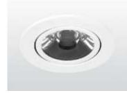
108 mm DIAMETER ROUND TRIM, RECESSED MOUNT WITH<br/>HIGH PERFORMANCE, LED DOWNLIGHT AND CLEAR GLASS<br/>LENS. 1000 NOMINAL LUMENS, MEDIUM ANGLE<br/>DISTRIBUTION AND IP20 RATING SUITABLE FOR DAMP<br/>LOCATION. .NON-INSULATED INSTALL TYPE, WHITE<br/>POWDER COAT FINISH.<br/>MODEL: LACS-120-L10-35K-CR80-W-RD-WH-DA2 OR<br/>APPROVED EQUIVALENT.<br/>VOLTAGE: 120V<br/>DRIVER: DIMMABLE<br/>LAMP: 10W LED 3500K (80 CRI)
