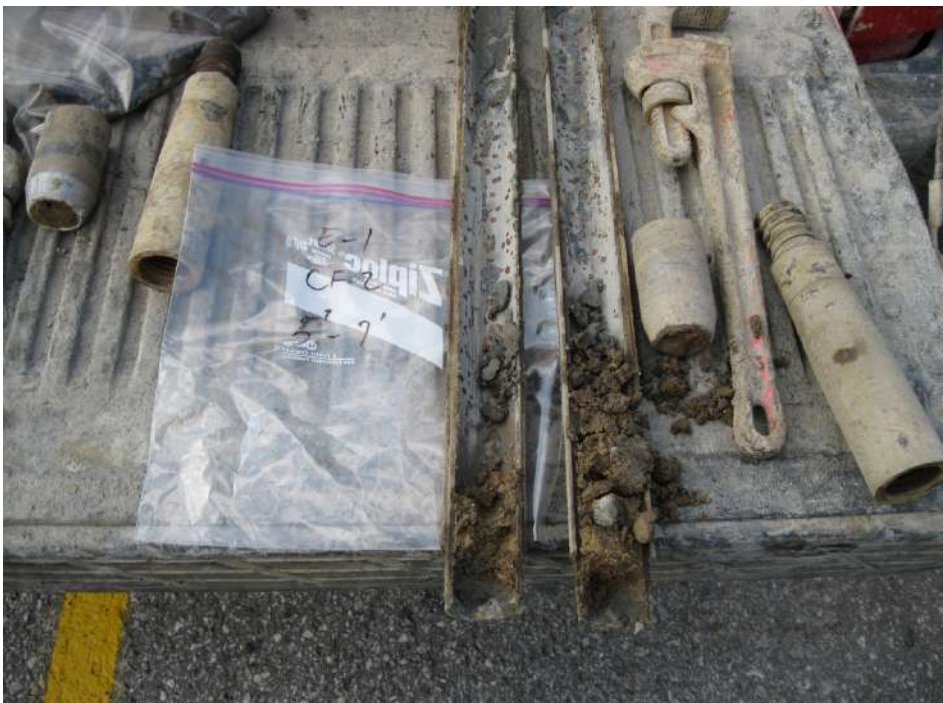
Typical sample of the backfill material (From borehole E-1)
